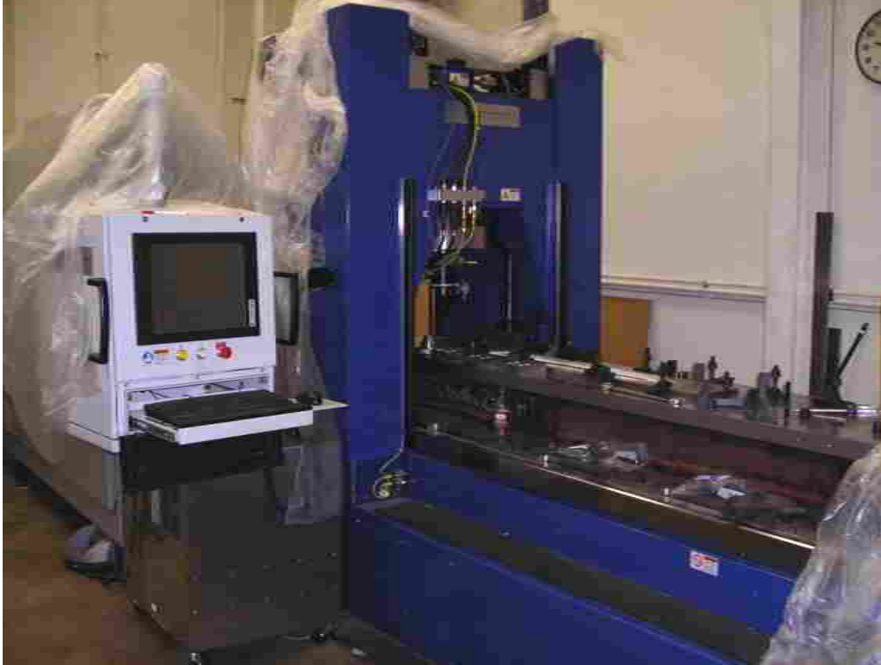
Figure 6 - Photograph of RM2 gantry style friction stir welding machine.
