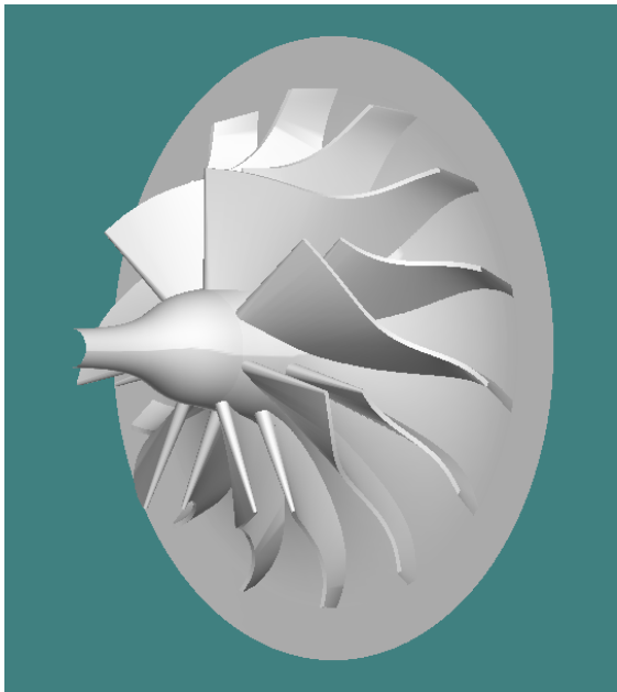
Figure 3-2 3-D illustration of the CCN30 impeller.
