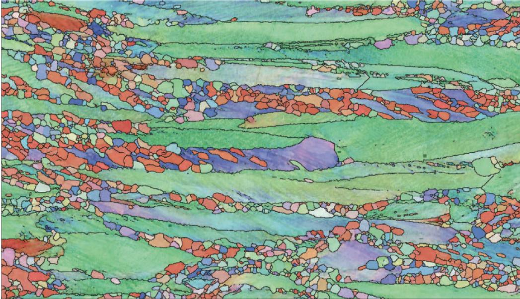
**Figure 1.1: Deformed and partially recrystallized iron aluminide illustrating non-equiaxed grain shapes and unequal grain size distributions often found in engineered materials (image courtesy of Oxford Instruments)**
