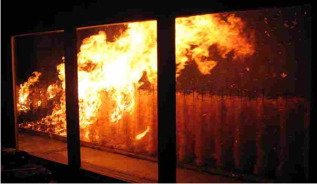
Figure 4.8. Photograph of fuel bed burned in the presence of wind at 2.2 m/s.
