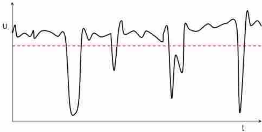
Figure 3-9: Signal of predominately high momentum fluid with occasional bursts of low momentum laminar flow resulting in negative skewness
