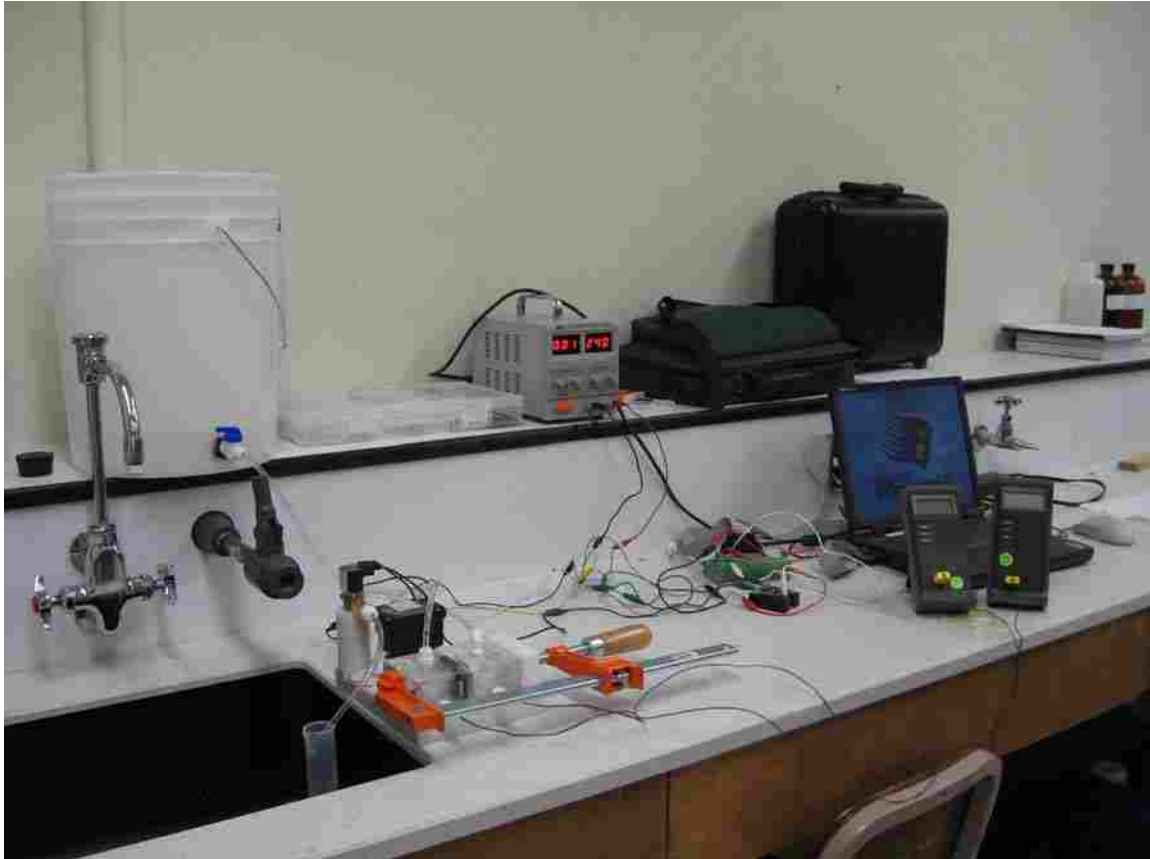
Figure 5-1: The complete test stand used to test the flow rates through the microchannels
