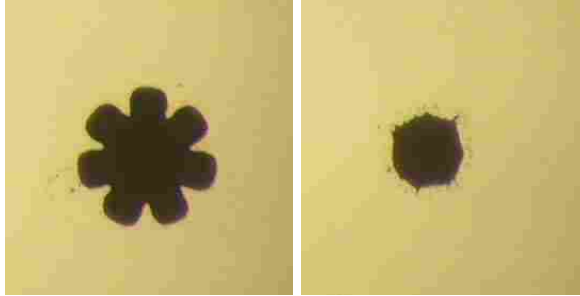
Figure 4-23: An optical microscope view of a typical 7-12 channel on the top surface (left) and on the bottom surface (right) of the wafer. These two pictures were taken at identical magnification.
