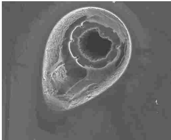
Figure F-2: When the photoresist for the second etch was spun on, it flowed around existing hole like water around a rock. Three levels can be seen here. The top level is the egg shaped hole that etched from the top surface during the second etch period. The second level is the last remnants of hole from the first etch period. This is estimated to be about 10 \mu\text{m} thick. The hydrophobic structures can still be seen along the perimeter. The third level is the rough walled circle in the middle. This is about 100 \mu\text{m} deeper than the initial etch so it reaches about 210 \mu\text{m} into the wafer substrate. It was etched during the second etch period.
