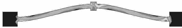
Figure 4.3: Finite-element-analysis displaying the stress distribution of PMT sensing flexures as they are displaced toward the top of the page.
