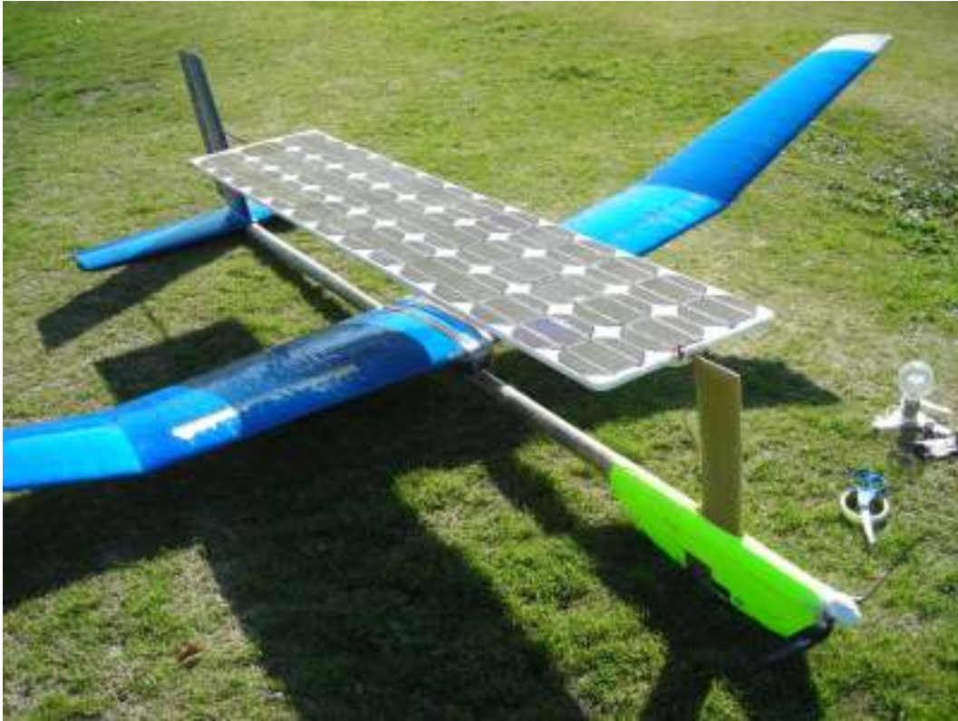
Fig. 4.1 NanSun’s assembled airframe, pictured with the solar tracking mode turned off and the horizontal panel mode turned on
