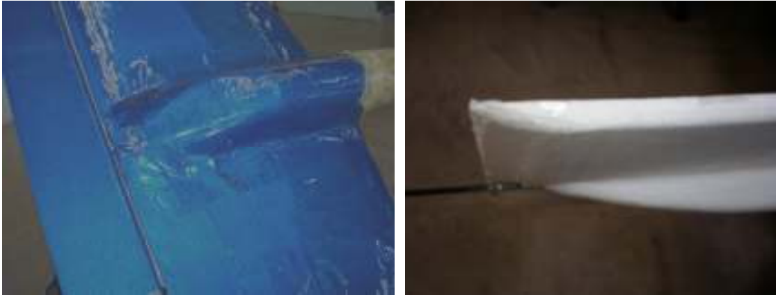
Fig. 4.2 The tail-fuselage junction (left) and the trailing edge of the solar panel (right) display how the members of NanSun were blended and shaped to minimize form drag and interference drag.
