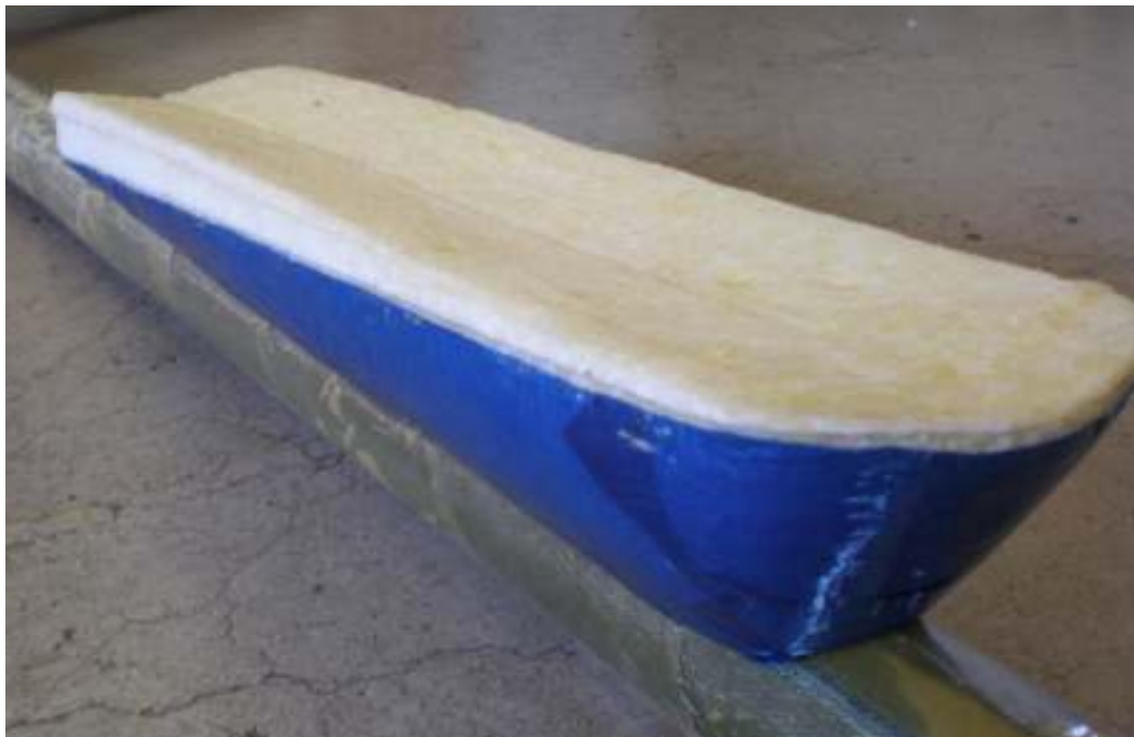
Fig. 4.3 NanSun's wing-setting piece on the fuselage
