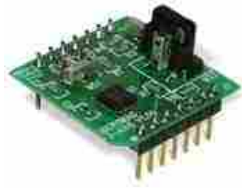
Figure 2.7: Above is the three-axis PNI magnetometer used in flight testing
