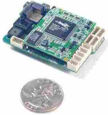
Figure 2.5: Above is the Kestrel autopilot that was used in flight testing.
