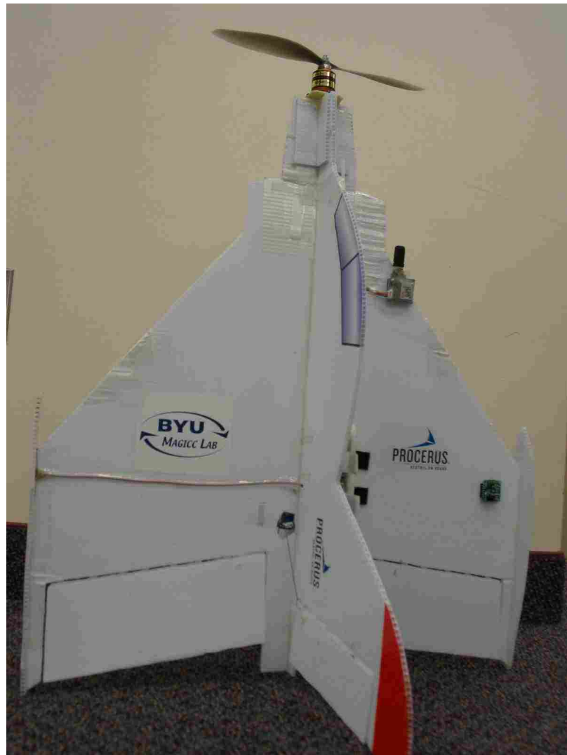
Figure 2.4: The tailsitter that was built to perform flight testing is shown.
