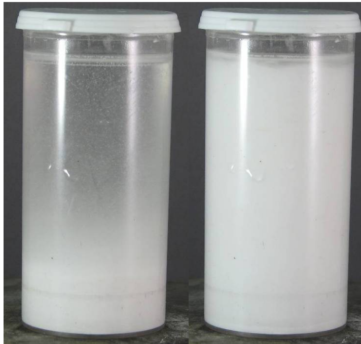
Figure 5.11 Slurry entrained by rotating magnetic bar: left, slow rotation; right, fast rotation
