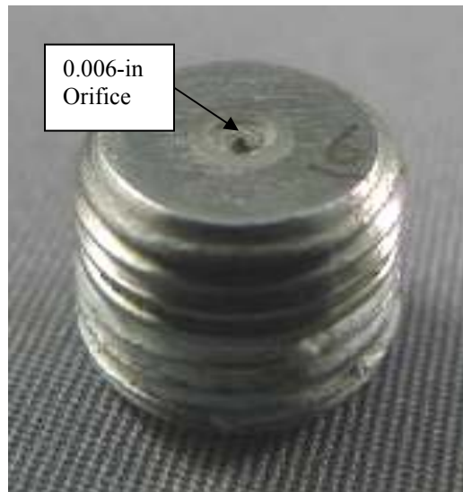
Figure 7.1 Nozzle with a 0.006-in diameter orifice in a sapphire disc
