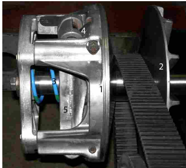
Figure 1-2 Primary Clutch: 1) moveable sheave, 2) fixed sheave, 3) spring, 4) weights, 5) spider.
