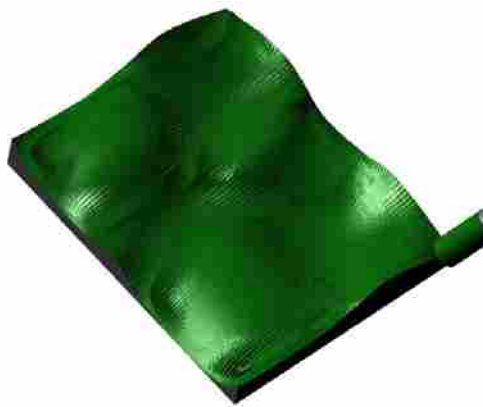
(e) Complex surface machined with the 3D C-space method.
