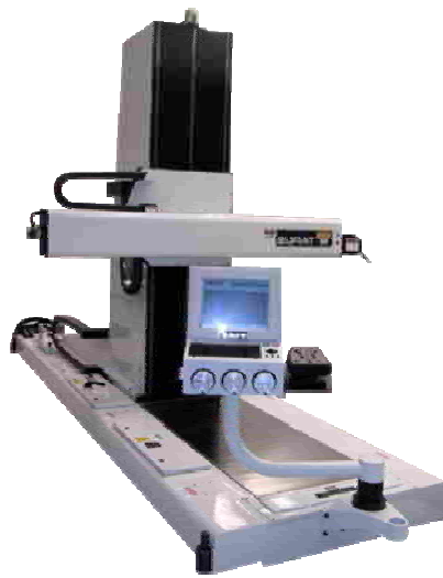
Figure 4-5 Five-axis full-size Tarus mill
