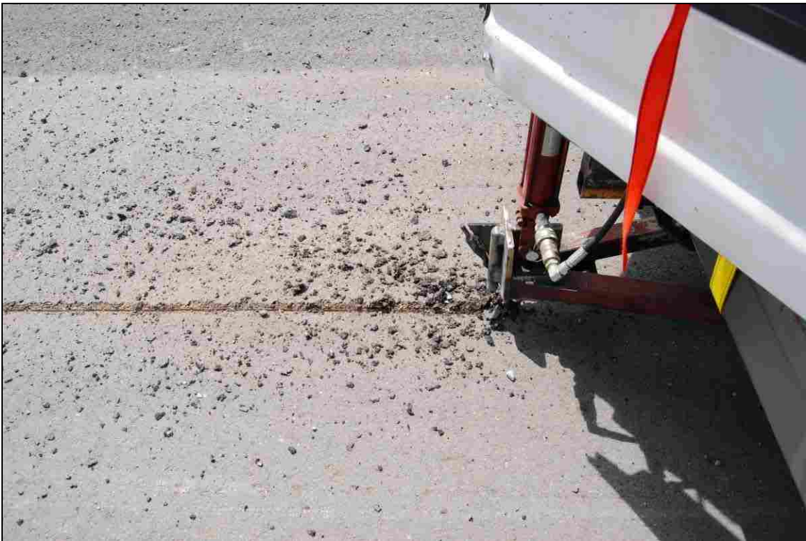
Figure 4.1 Post-test roadway gouge
