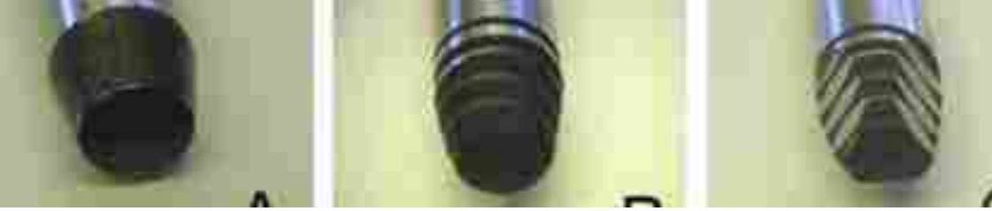
Figure 2-2: Existing Probe Geometries [3]
