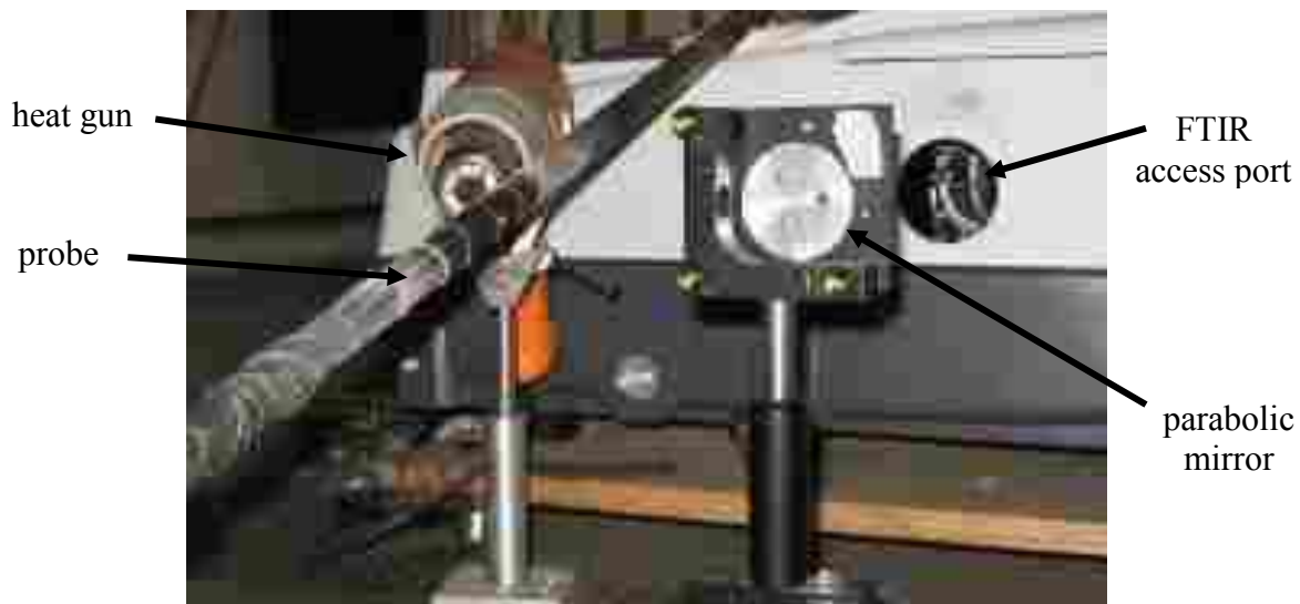
Figure 6-7. Experimental setup used to measure the spectral emittance of the clean, painted deposit probe.
