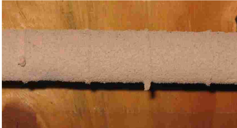
Figure 3-6. Typical ash deposit on the probe after a deposition experiment.
