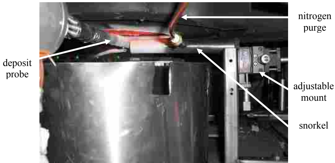
Figure 6-14. Experimental setup for measuring emittance of ash deposits that form in a reducing environment.
