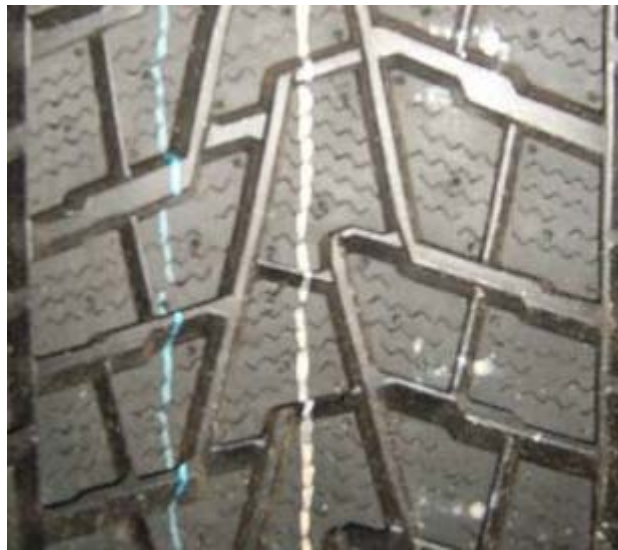
Figure 4-5 Snow tire with siping and very complex geometry
