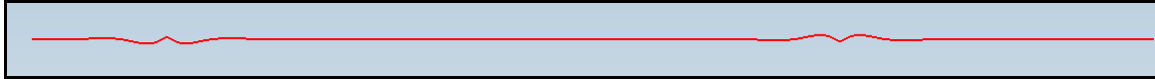
Figure 4-6 Test Case 5: Linear tool path of ideally zero curvature with two noisy points. Points are both 0.2 mm away from straight line and form ripples that almost reach 0.4 mm from straight line. These noisy points create sections of high-curvature ripples. The NC tool will decrease feedrate from ideal to maneuver high-curvature ripples.
