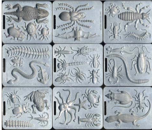
Figure 2-6 Molds for children’s toys that contain very high-curvature. Curvature of molds could be slightly reduced without affecting their quality.
