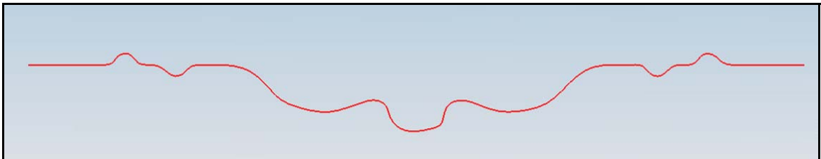
Figure 4-1 Test Case 1: Tool path with many low curvature radii. Tool path is fairly smooth and long. NC controller will decrease the feedrate through these low curvature sections, but not significantly.
