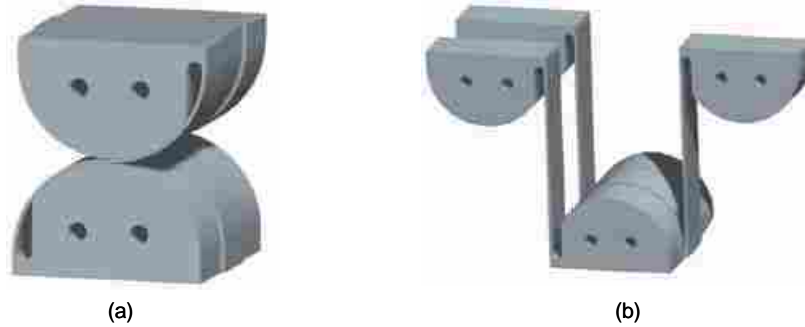
Figure 2.21 The Compliant Rolling-contact Element (CORE) in its assembled configuration (a) and pre-assembly (b) [28].
