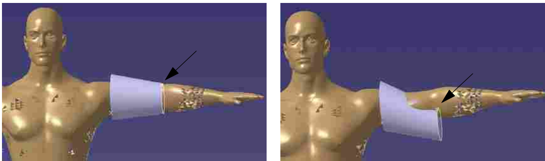
Figure 4.9 Regeneration of a Blend as a Reference Point is moved.
