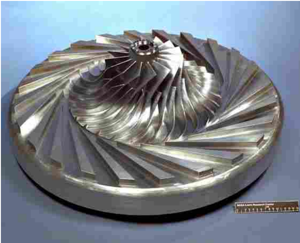
Figure 1-2. Picture of a wedge diffuser build with the shroud removed to show the impeller and diffuser. A short vaneless diffuser, or vaneless space, is located just after the impeller exit [3].
