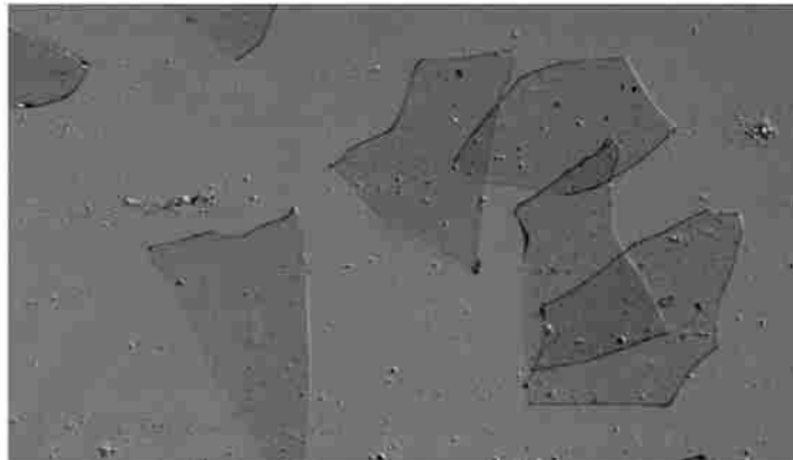
Flakes 180-212 \mu m Sieved Twelve Times
