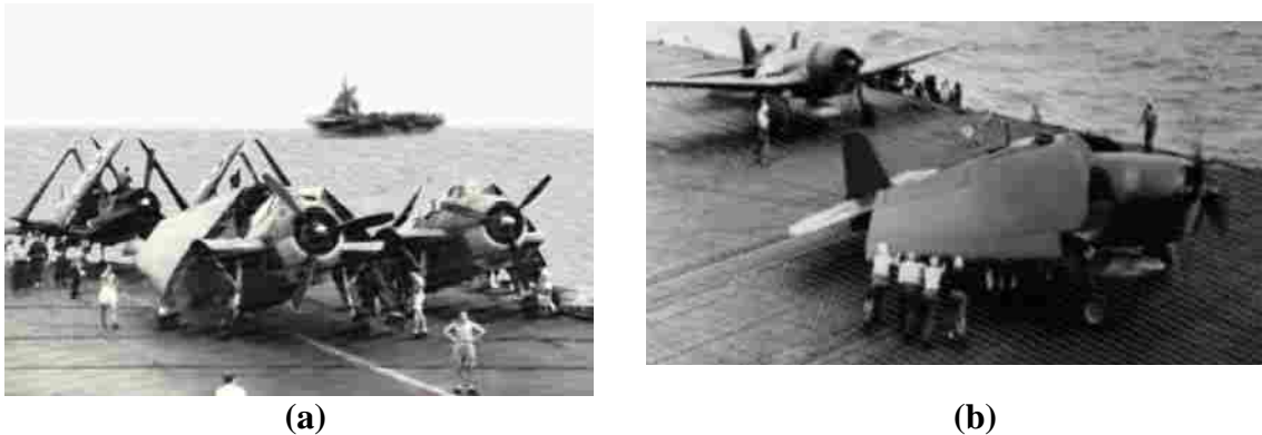
Figure 2-6. (a) USS Formidable, with Vought Corsairs behind and Grumman Avengers in the foreground, 1945. (b) Folding the wings back on a Grumman TBF Avenger, 1944. [12]
