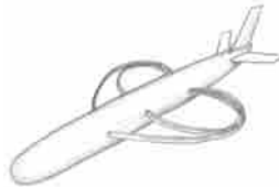
Figure 4-13. All motion for this bent-back wing occurs within the original wing plane.
