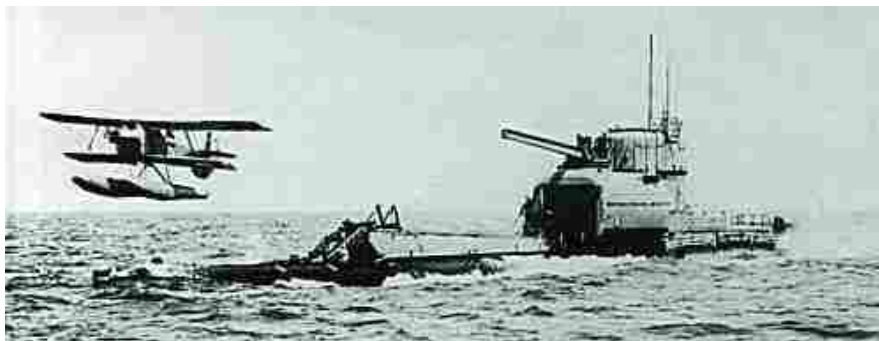
Figure 2-8. The M2 submarine, just after launch of the Peto biplane fighter. [13]
