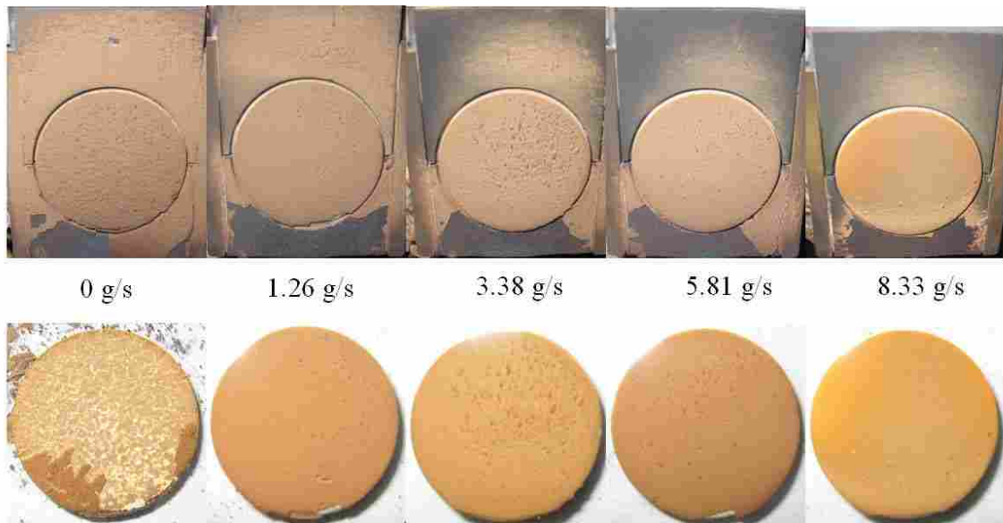
Figure 5-1: Coal impingement cooling series post-test buttons immediately following shutdown (top) and after cool down to room temperature (bottom)
