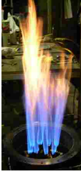
Figure 2-5: Modified flame holders in operation (cone removed)
