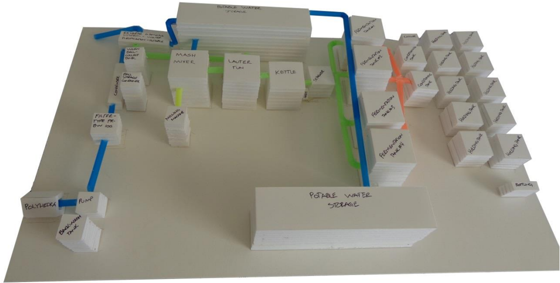
Figure 12 – Systems Model. This model portrays the various systems involved in the project. The volumes are proportioned accordingly and arranged in an efficient layout. Note: This model was made and photographed by Ryan Luczkowiak.
