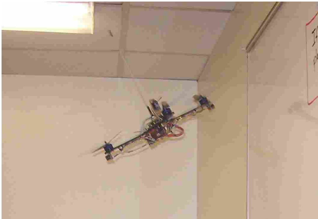
Figure 6-4: The quadrotor in flight near a wall to generate large feedback forces
