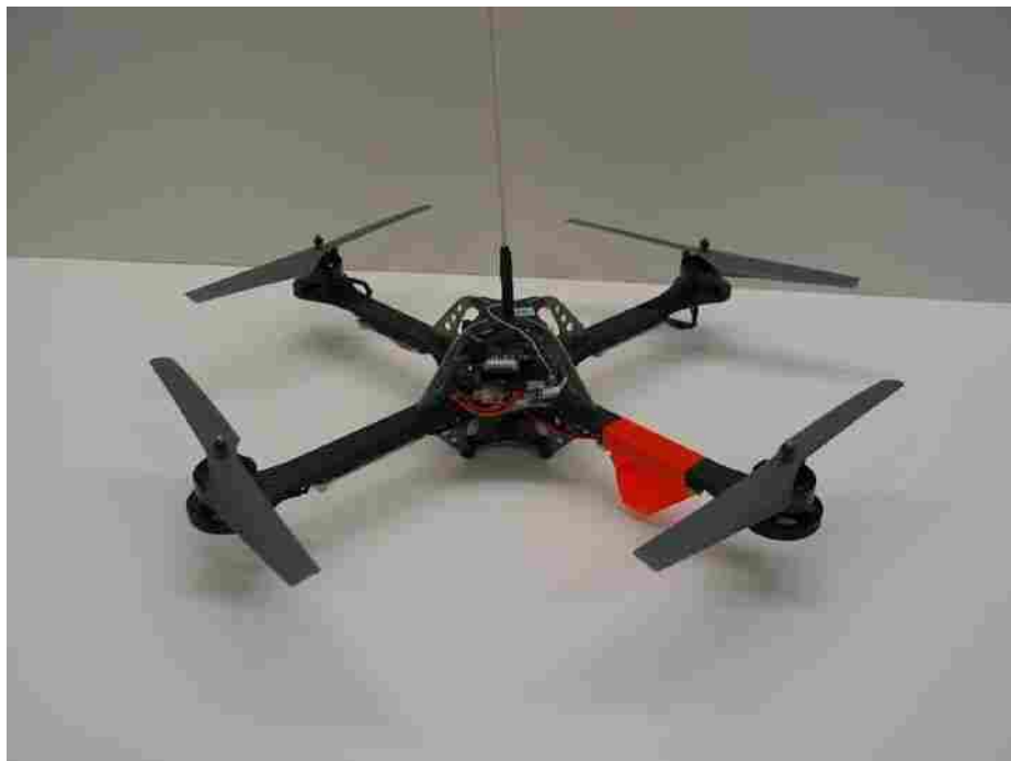
Figure 1-1: A typical quadrotor with four coplanar rotors around the main body that houses the battery and computing hardware. This quadrotor does not have a camera.
