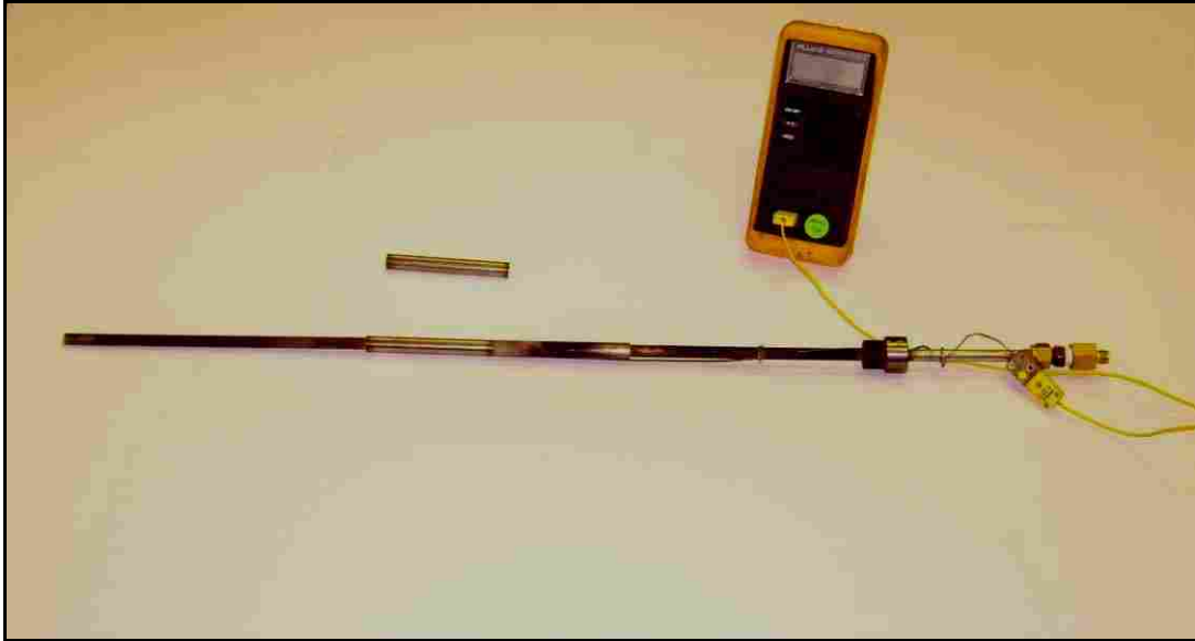
Figure 4-2 Cooled deposition probe used to simulate a superheater tube in cross flow. The probe features a 1.2 cm diameter by 10 cm long sleeve that can be removed to allow for easier measurement of the deposited mass
