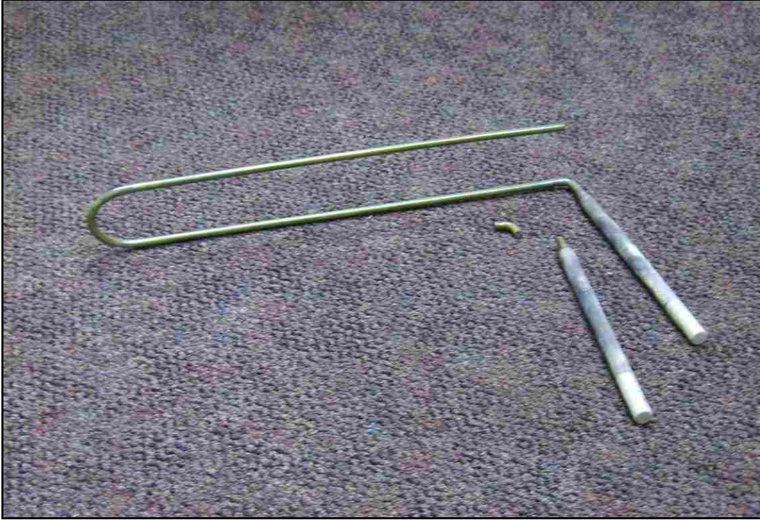
Figure A-12 - Broken heater element.
