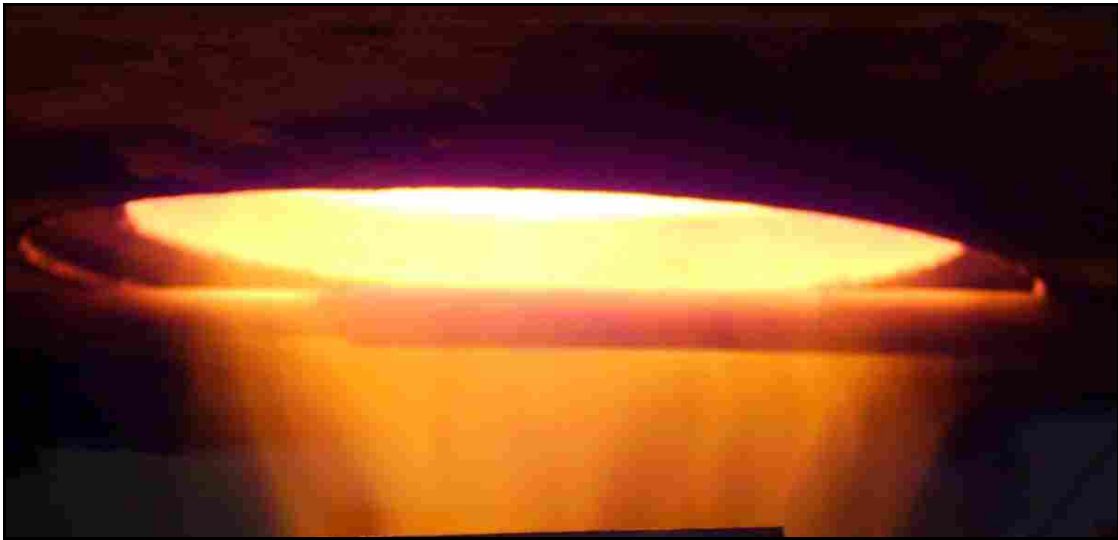
Figure 4-4 Typical deposition experiment showing the deposition probe in place under the coal- and natural-gas-fired reactor.
