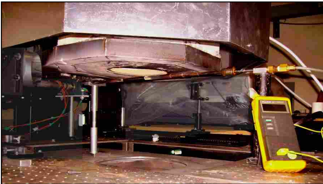
Figure 4-3 Deposition probe installed 2.5 cm below the bottom of the reactor.
