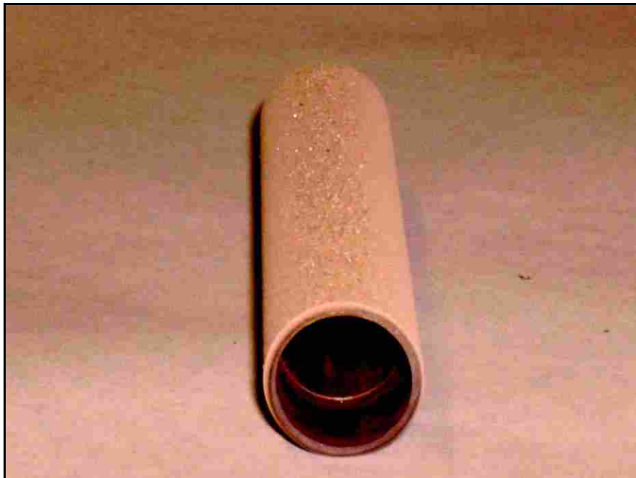
Figure 4-5 Thin deposit layer formed on the probe's deposition sleeve. Note that the sleeve has been removed from the rest of the probe so that the deposit can be weighed and collected.
