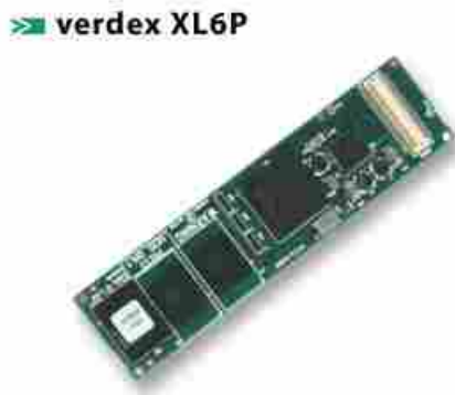
Figure 3.2: Gumstix Processor: The Gumstix processor is a very small Linux computer. Weighing just 2.5 oz., it provides enough processing power to perform moderate computer vision calculations.
