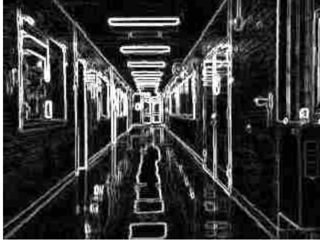
Figure 4.2: Gradient Magnitude Image From the Sobel Edge Detector: The image gradient magnitude brings out strong edges. This image is the result of using the Sobel kernel to estimate the pixel gradient.
