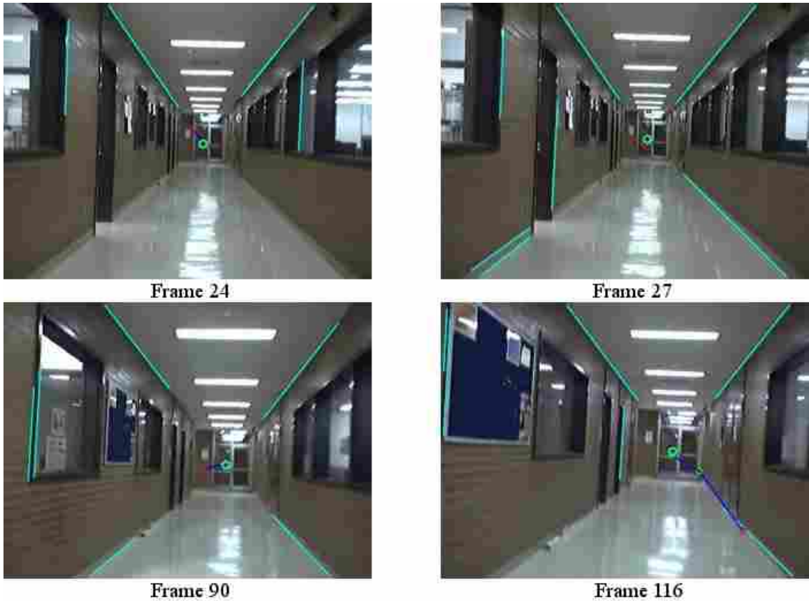
Figure 4.11: Burns Line Detector Successes: The Burns Line Detector was able to detect the vanishing point in many of the frames, even if the prior vanishing point discovered erroneously, as shown in Frame 116.
