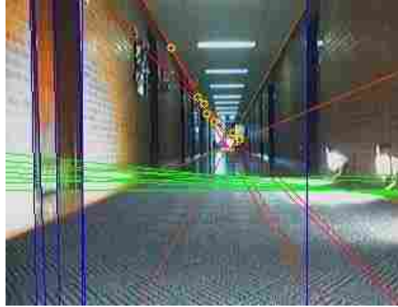
Figure 4.13: Finding All Vanishing Points: Hough Transform Method of Finding all vanishing points
