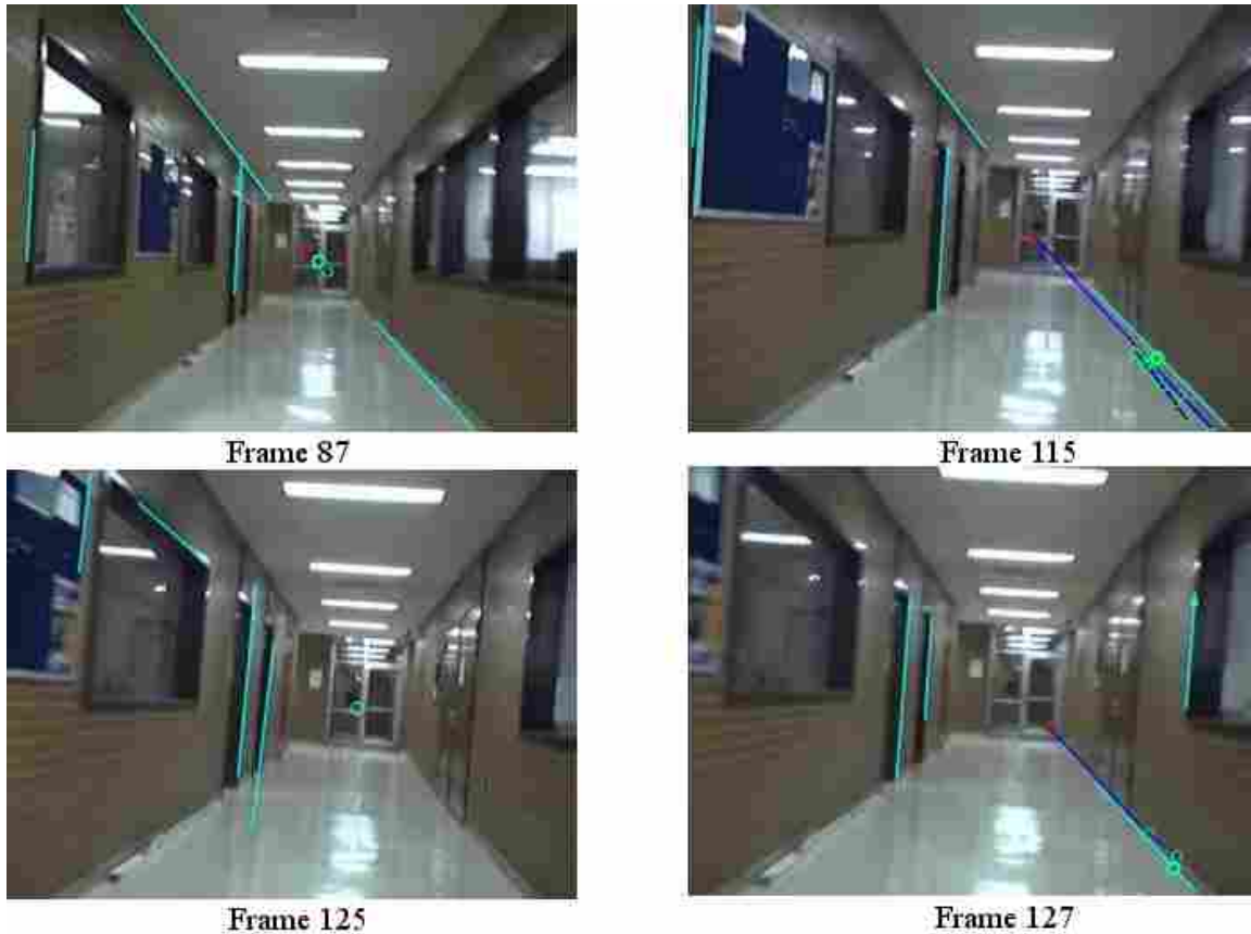
Figure 4.12: Burns Line Detector Failures: If the number of lines found from the Burns Line Detector was insufficient, the Leveburg-Marquadt algorithm converged incorrectly.
