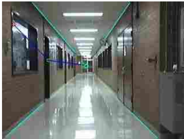
Figure 4.8: Example of Vanishing Point Detection: Here, the vanishing point is detected using the Levenburg-Marquadt algorithm. The approximation to the Hessian quickly drives the estimate of the vanishing point to the optimum location.
