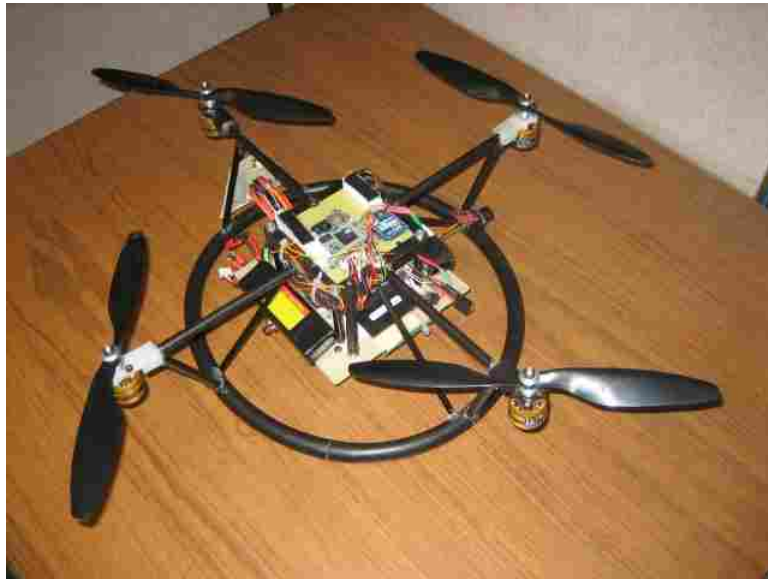
Figure 1.1: Quadrotor Helicopter: The quadrotor helicopter is the primary vehicle used in this research. It is capable of sustained hover flights and of holding substantial payloads.
