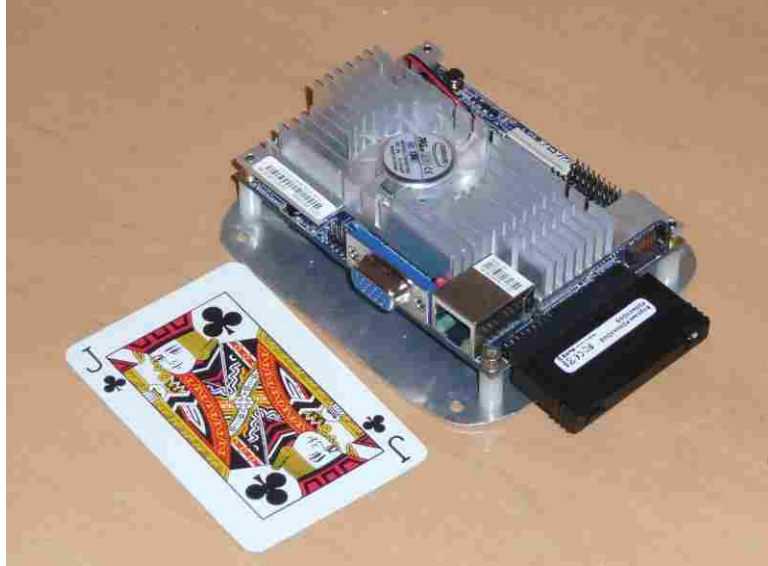
Figure 3.3: Pico-ITX Processor Board: The Pico-ITX form factor computer provides a substantial amount of processing power in a very small size. Running Ubuntu Linux, it is capable of running computer vision algorithms in real-time and of interfacing to remote computers over wireless remote desktop connections.
