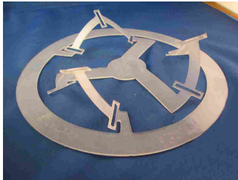
Figure 3.14: The actuated position of a LET Joint used in a spherical mechanism.
