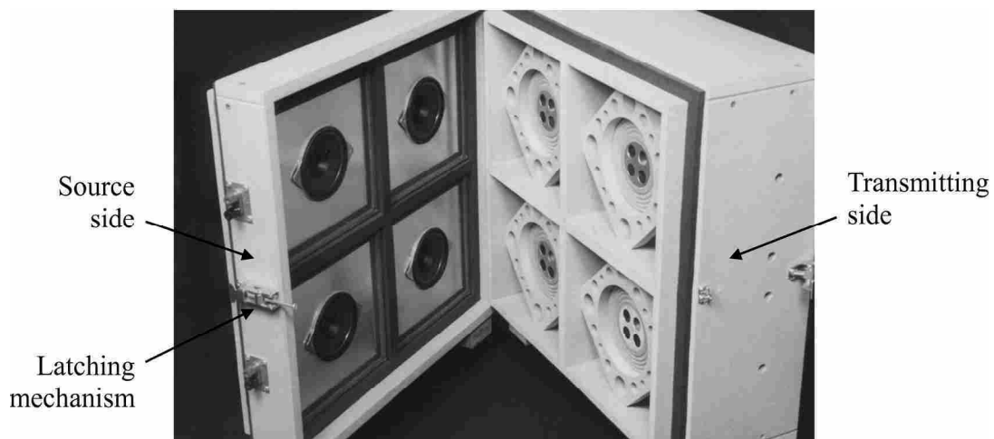
Figure 3-1. Photograph of Leishman's ASP array. Photographs reprinted with permission from [48]. Copyright 2005, Acoustical Society of America.
