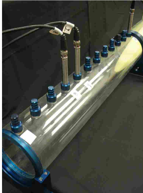
Figure 6-5. Photograph of the receiving-side tube of the measurement apparatus. The microphone ports are spaced 5 cm apart and the tip of the anechoic wedge is visible in the upper right.
