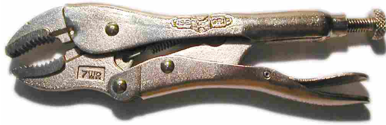
Figure 2.1: Self-locking pliers composed of a rigid-body force-multiplying mechanism
