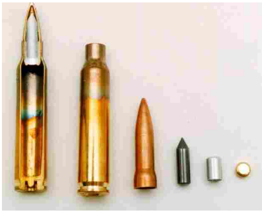
(a) Disassembled M993 7.62mm NATO standard armor-piercing round [15]
