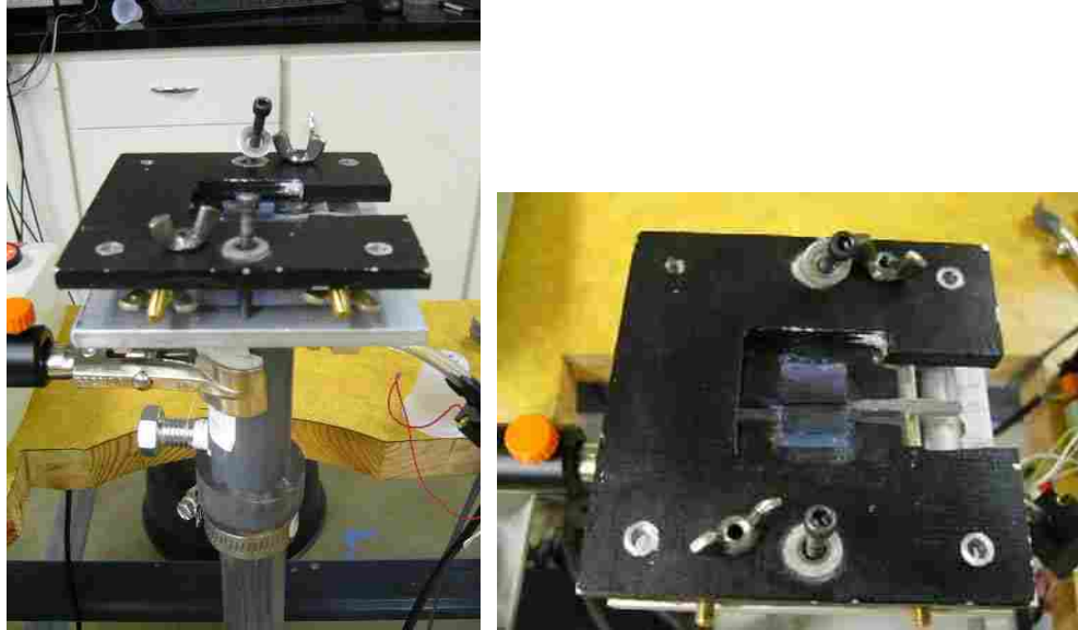
Figure 3-4 Test Fixture A with sub-glottal tube attached (seen at left as PVC tubing).
