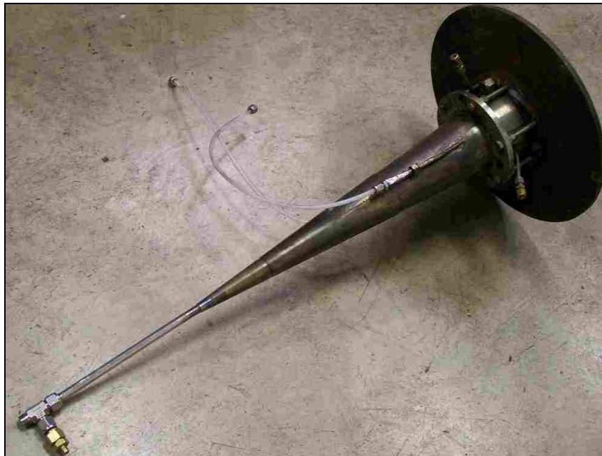
Figure 13. The cone and burner exterior. Coal and primary oxidizer enter through the stainless steel connection at the bottom left of the photograph. Natural gas enters through the brass fitting to the lower right of the stainless steel connection. The white plastic tubing is for water cooling of the burner face. All other fittings are no longer in use.
