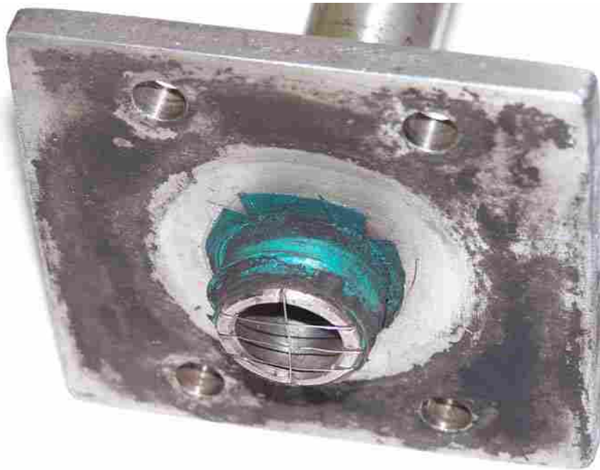
Figure 11. Outlet of the coal feeder auger pipe showing four fine wires crossing the opening.
