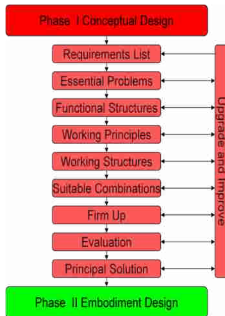
Figure 3.1 Conceptual Design Process
