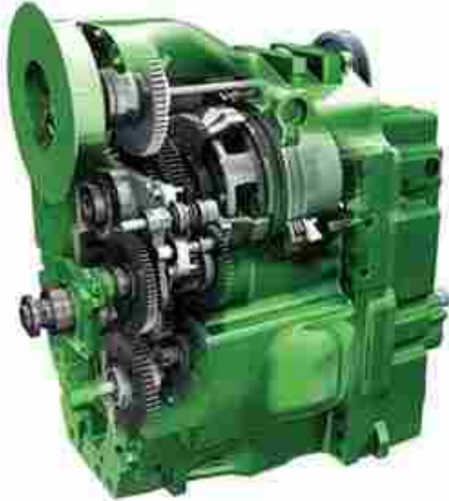
Figure 2.18: John Deere IVT (Taken from http://www.deere.com/en_AU/equipment/ag/tractors/8030_series/transmission.html )
