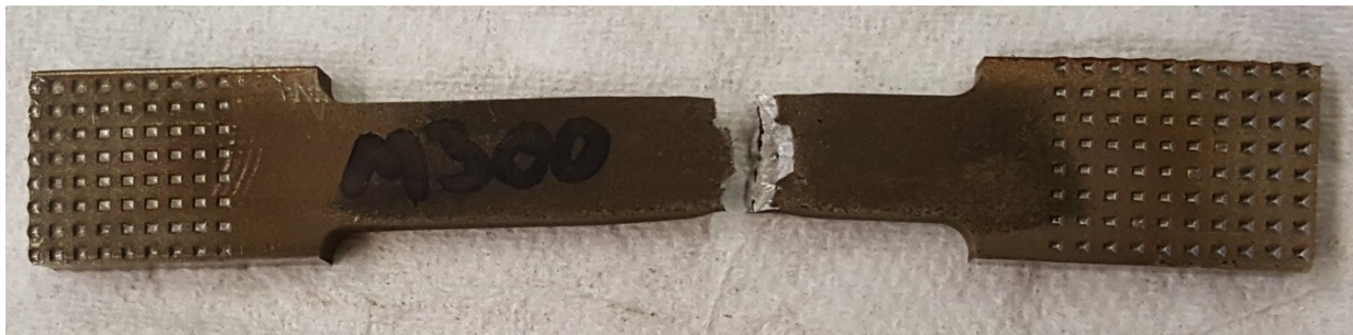
Figure 4-41: Fully Additive DED M300 Tensile Specimen Post Break
