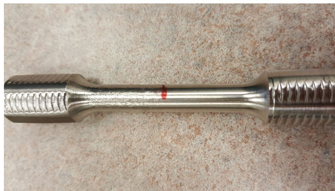
Figure 4-10: Hybrid SS316L Torsion Specimen Post Twist
