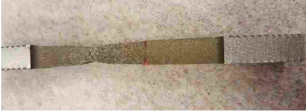
Figure 4-17: Hybrid SS316L Tensile Specimen Post Test
