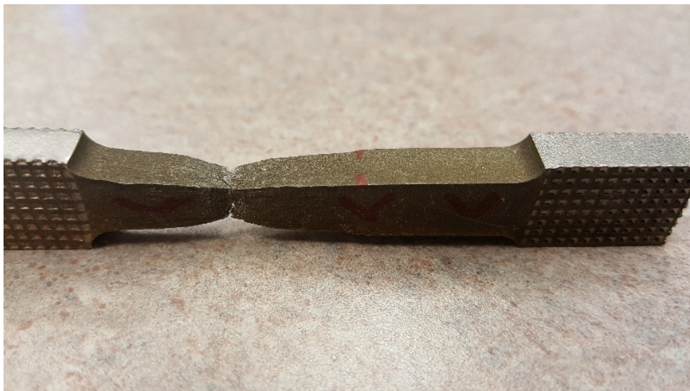
Figure 4-18: Hybrid SS316L Tensile Specimen Post Test
