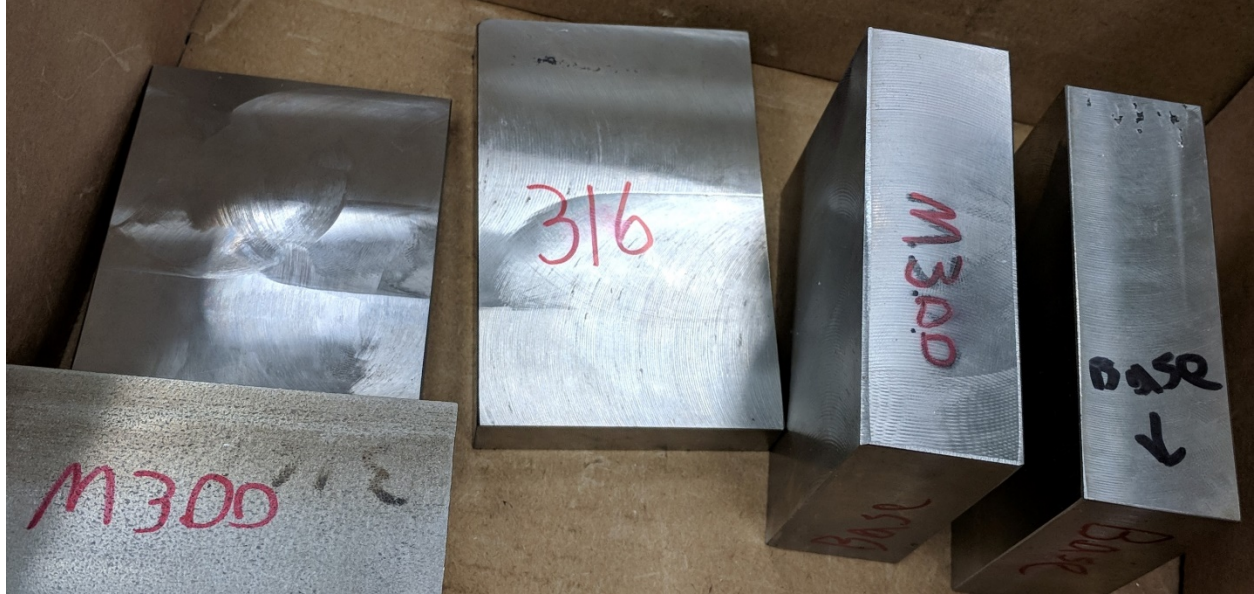
Figure 3-1: Fully Additive and Hybrid SS316L and M300 Samples via DED
