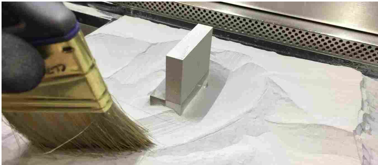
Figure 3-3: View of Specimens in Powder Bed of 400W EOS M280
