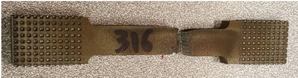
Figure 4-48: Fully Additive DED SS316L Tensile Specimen Post Break
