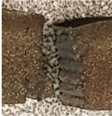
Figure 4-49: Close-up View of Fractured Surface in DED SS316L Tensile 1
