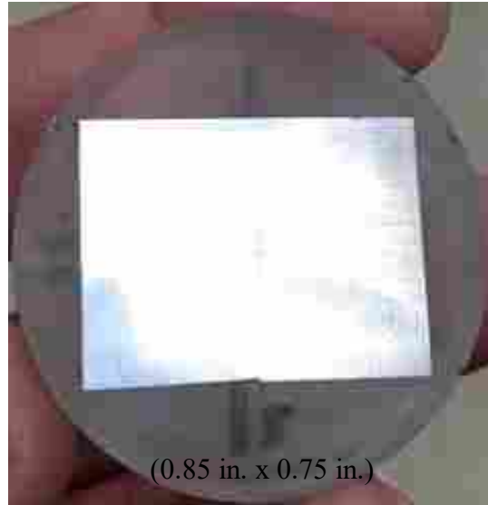
Figure 3-14: SS316L Specimen Ready for Polishing
