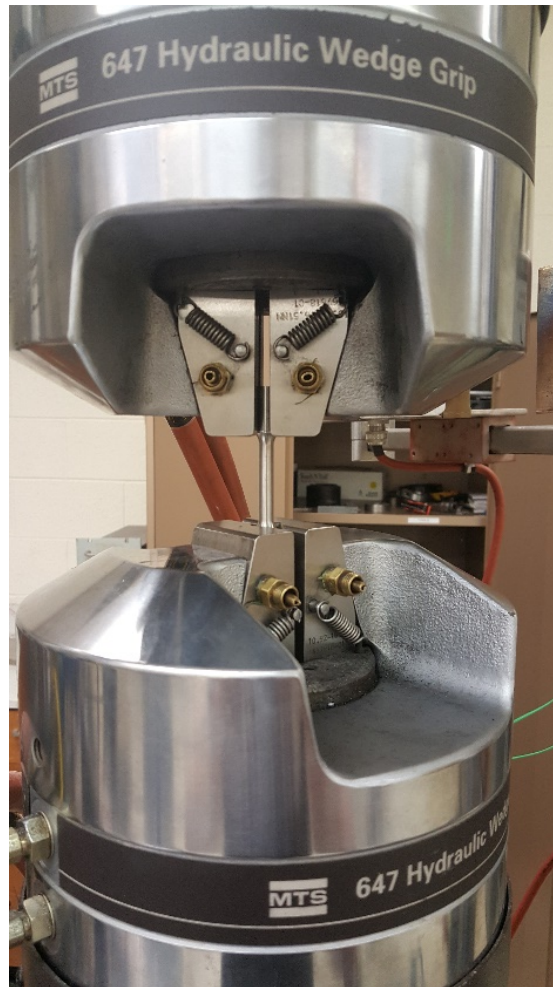
Figure 3-6: Torsion Specimen in Instron
