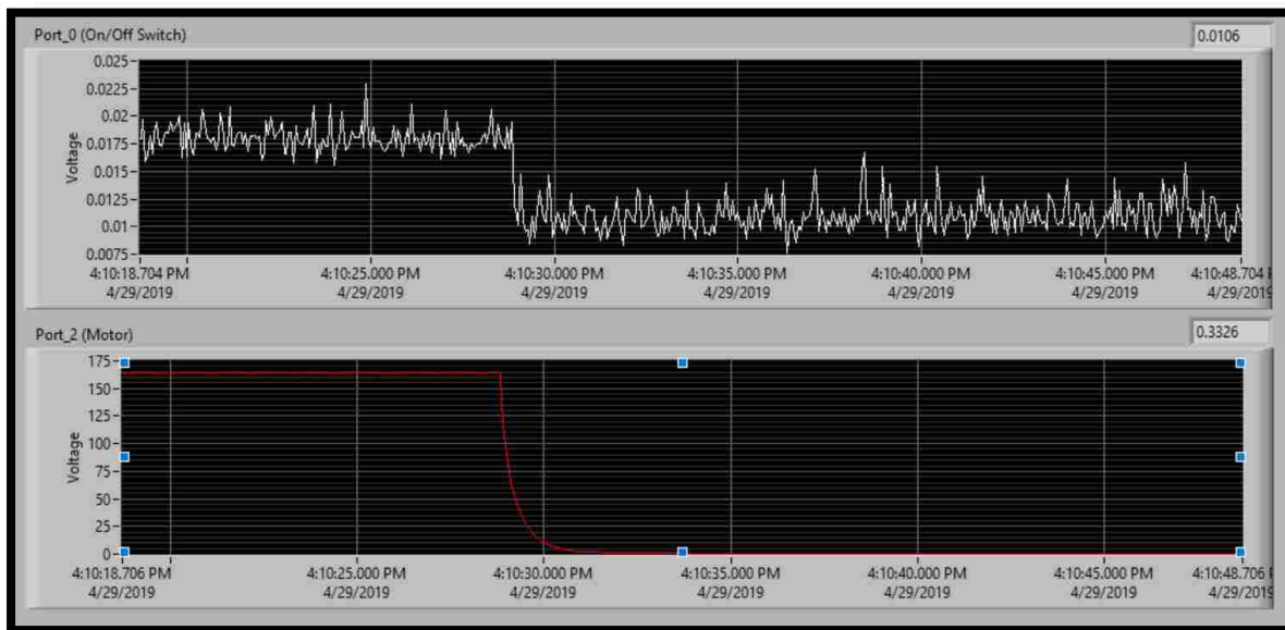
Figure 4-20: Lathe_11 Running, then Motor Lever Switched Off
