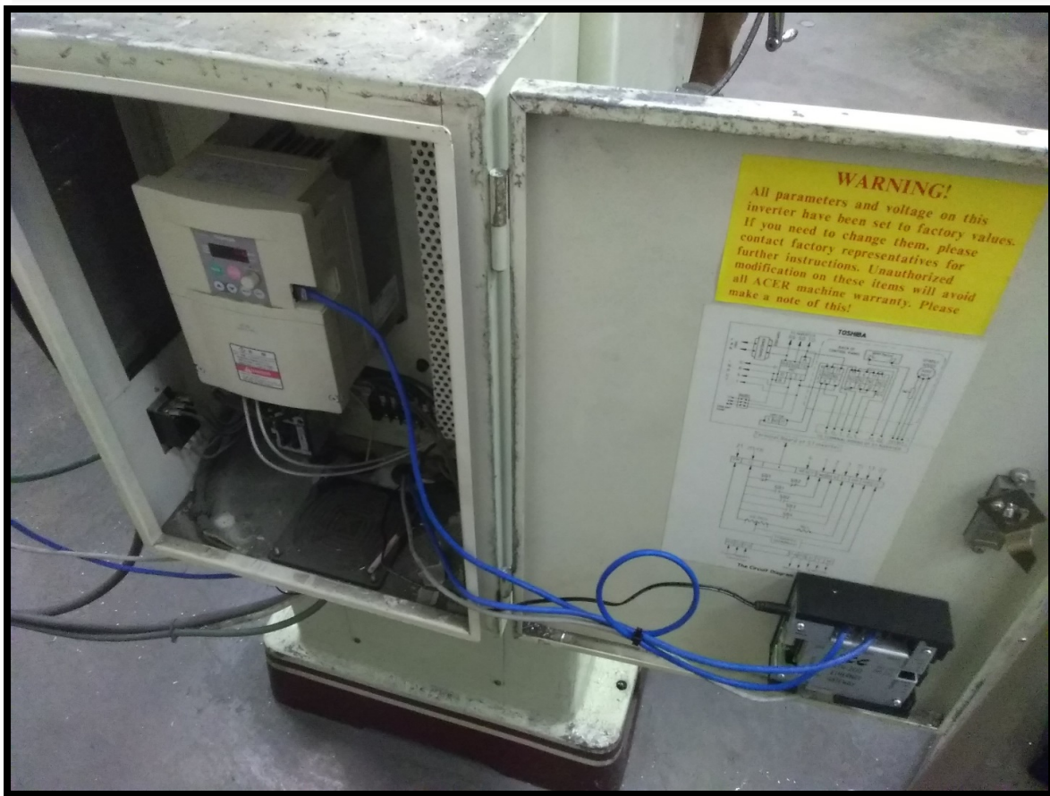
Figure 3-7: Communication Connection Between the Mill and KEPServerEX
