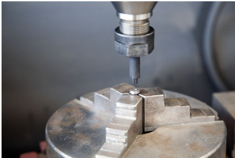
Figure 4-4: Graphite Electrode Positioned to Plunge a Torx Pocket in a "Blank"
