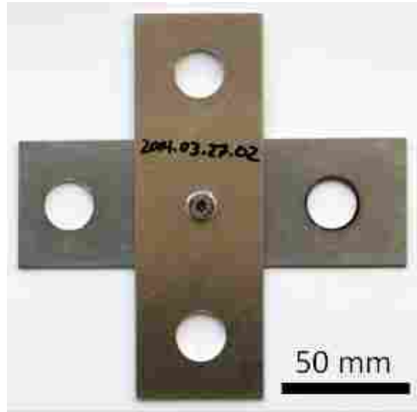
Figure 4-64: Typical Arrangement of Cross Tension Test Coupons
