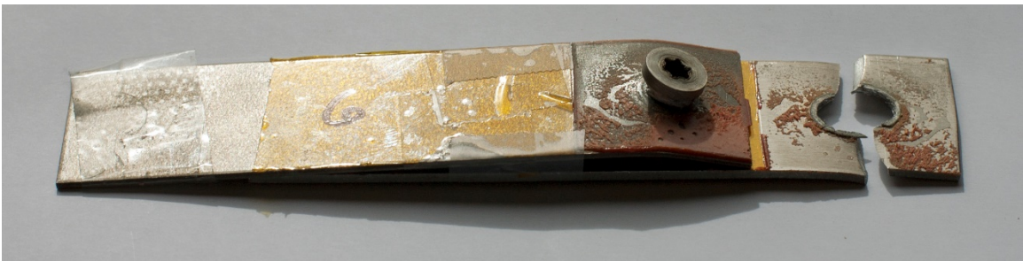
Figure 4-55: Hybrid Specimen with Aluminum Failure
