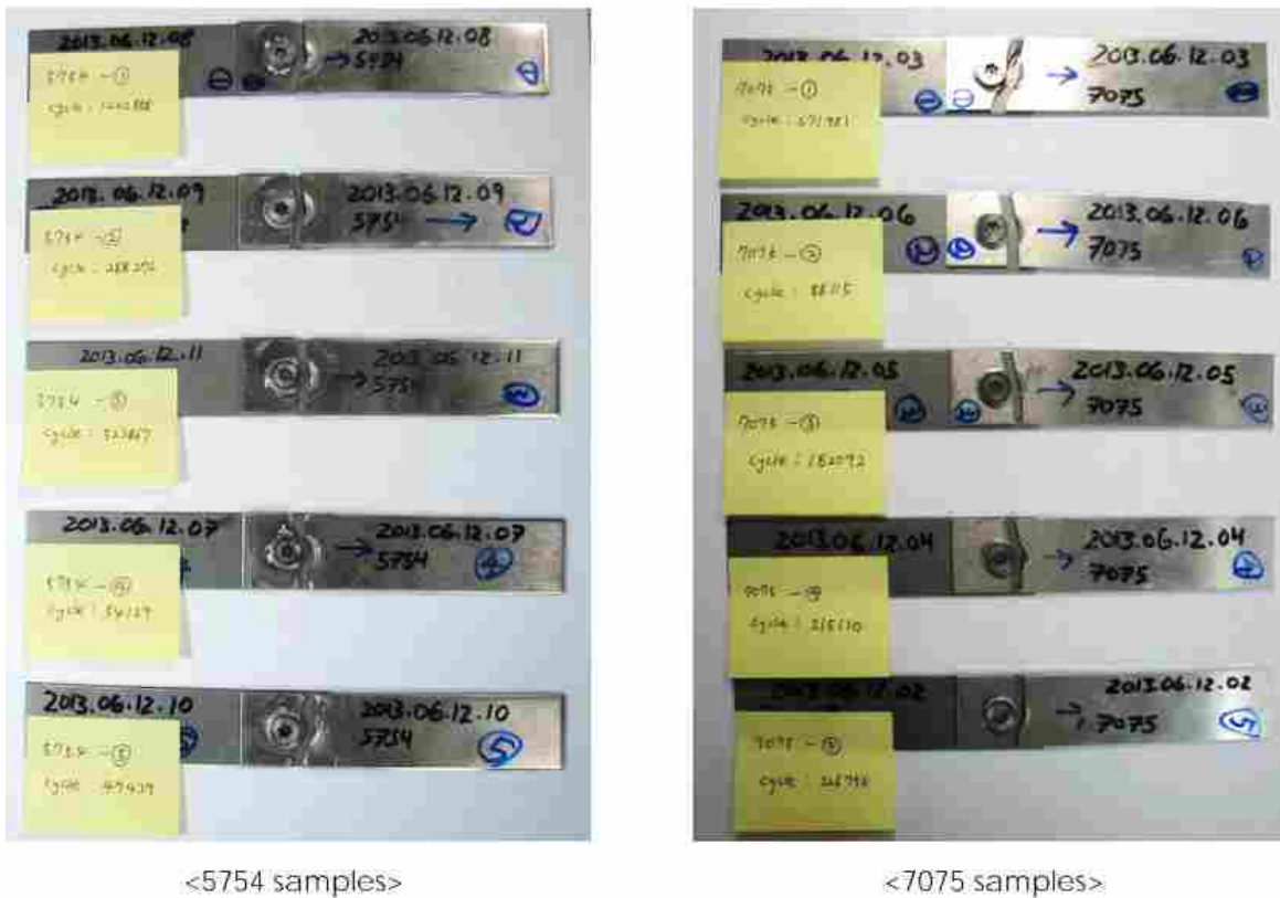
Figure 4-47: All Samples Tested in Fatigue Cycles, with Material Failure in Every Case
