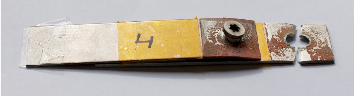
Figure 4-53: Hybrid Specimen with Aluminum Failure
