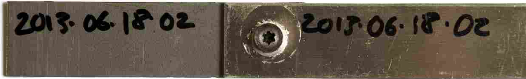
Figure 4-10: Typical Lap Shear Specimen, With ID Number
