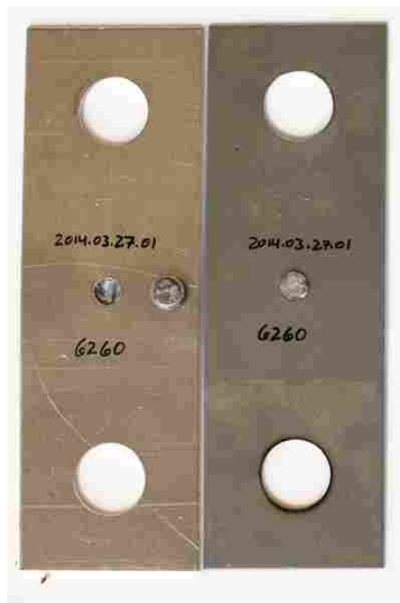
Figure 4-66: Specimen Tested in Cross Tension, Exhibiting Bit Head Failure
