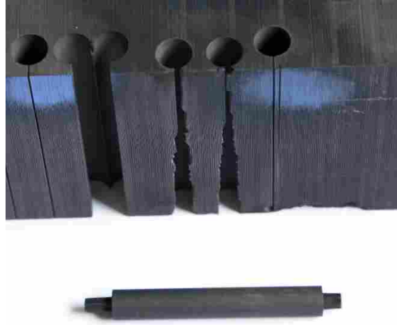
Figure 4-3: Graphite Cylinder Cut From a Block Using Wire EDM
