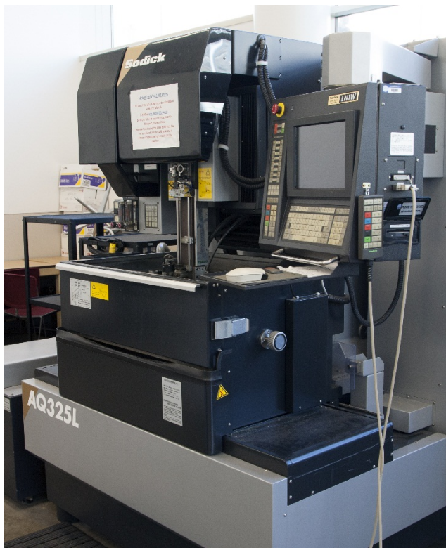
Figure 3-9: Wire EDM Machine Used to Section Samples and Create Tooling
