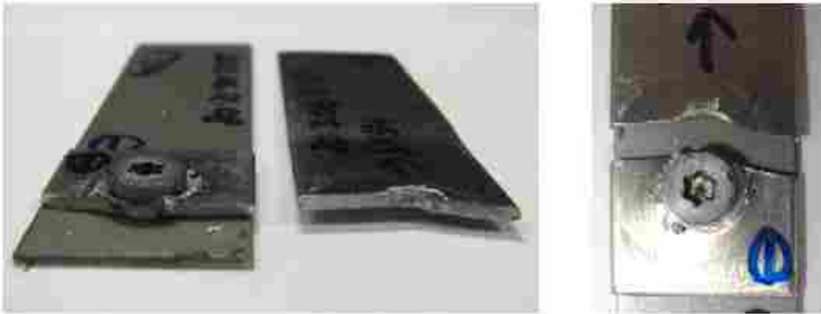
Figure 4-48: Fatigue Specimens with Fractured Aluminum and FBJ Bond Intact
