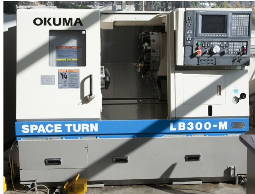
Figure 3-4: Okuma Space Turn CNC Lathe Used for Experimental Work
