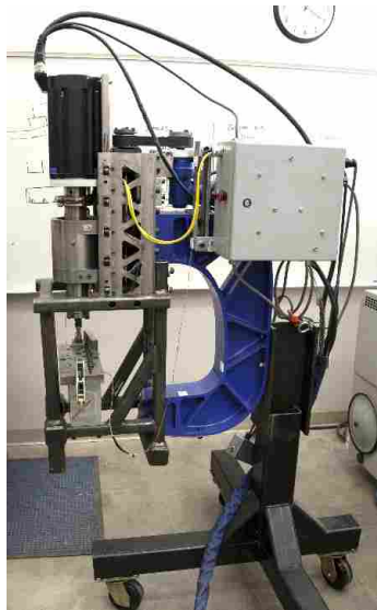
Figure 3-1: Friction Bit Machine at BYU
