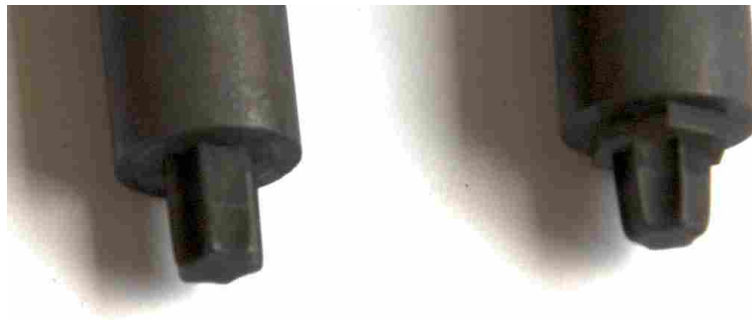
Figure 4-5: Graphite Electrodes Showing Various Degrees of Erosion
