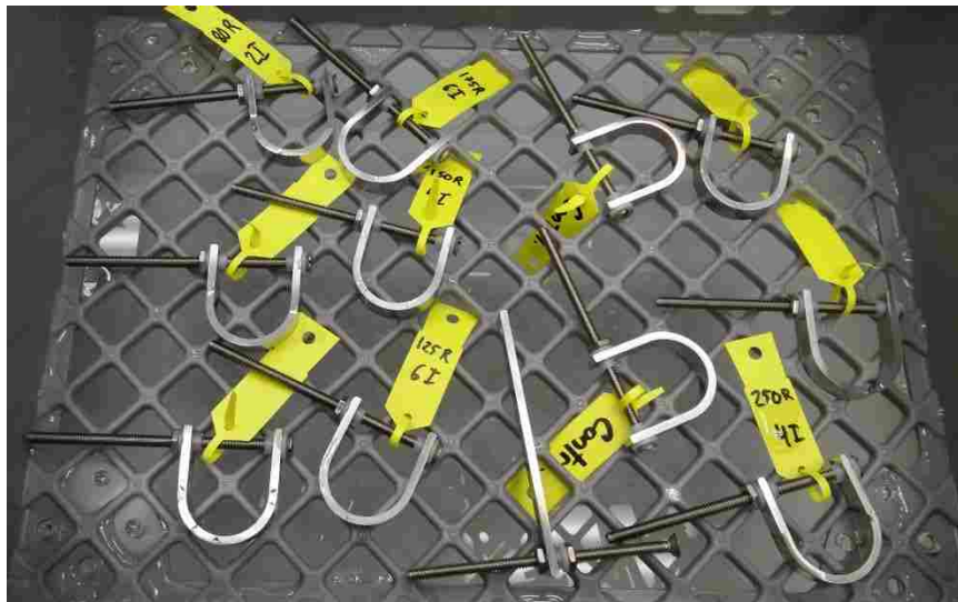
Figure 3-10: Corrosion Testing Specimens in Basket
