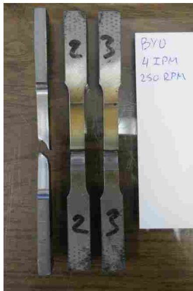
Figure 4-6: Tensile Failure of Z-Depth Control Specimen 4I-250R
