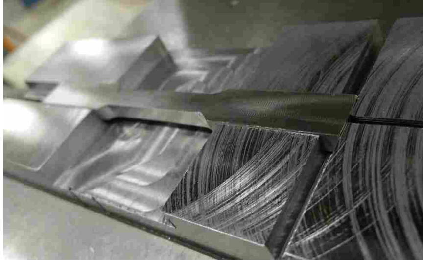
Figure 3-2: CNC-Machined Dogbone in Custom Fixture
