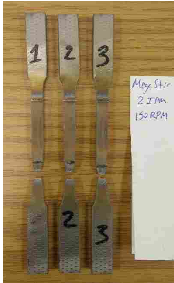
Figure 4-7: Tensile Failure of Z-Force Control Specimen 2I-150R
