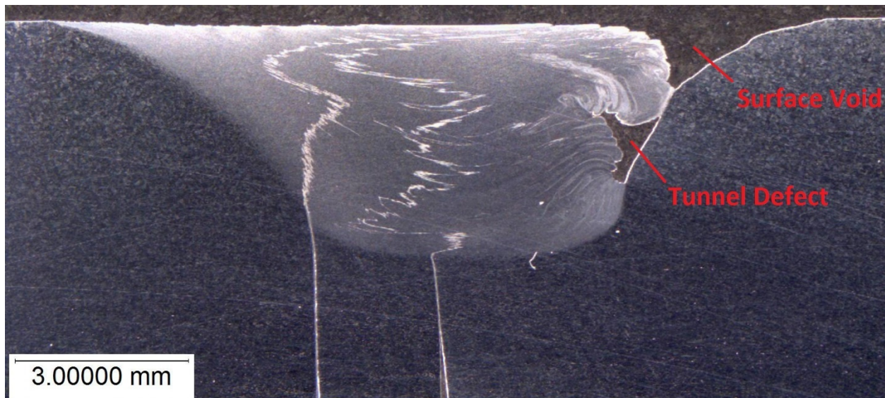
Figure 4-16: SCH1 – Example of Surface Void and Tunnel Defect
