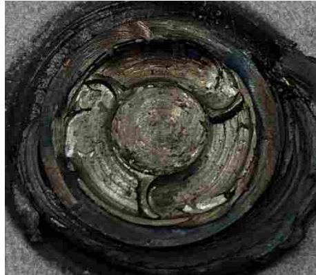
Figure 4-38: Severe Smearing of Drive Features During Experiment
