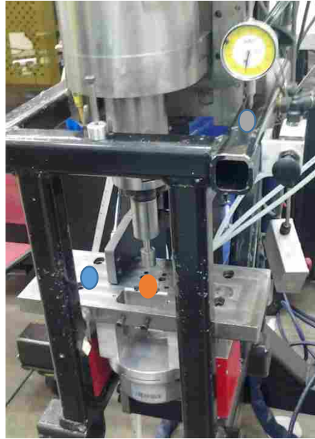
Figure 4-2: FBJ Machine Points of Deflection Measurement
