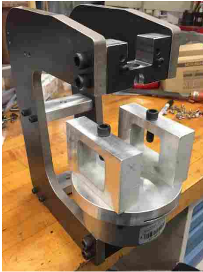
Figure 4-3: Pneumatic Clamp Before Installation on the FBJ Machine
