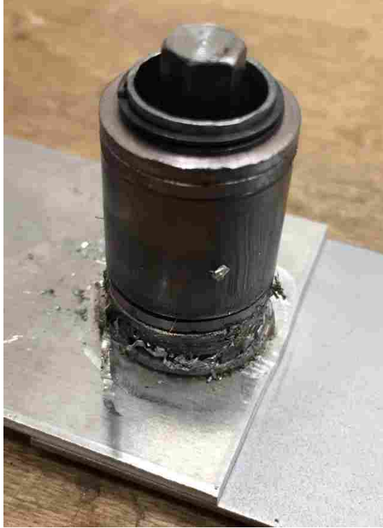
Figure 4-26: Torx Plus Driver Welded to Bit
