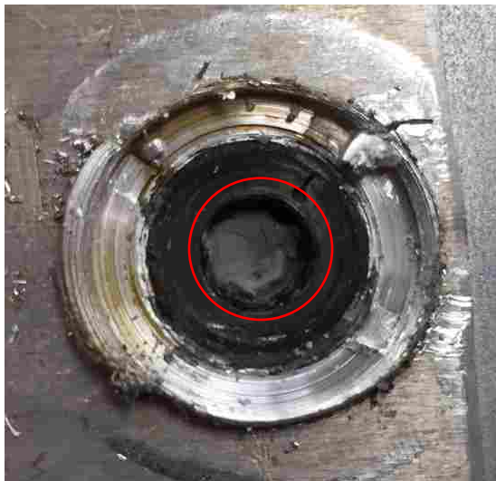
Figure 4-27: Fracture After Removing Welded Driver from the Bit
