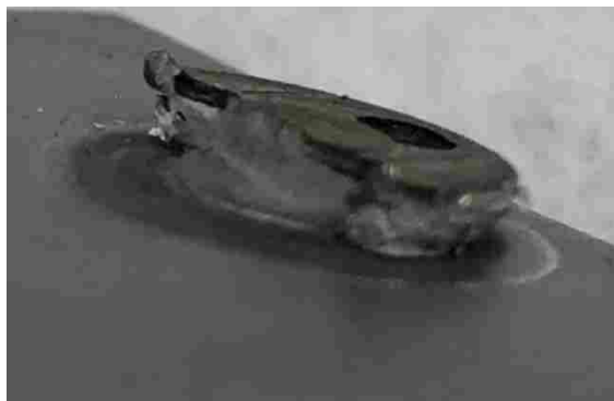
Figure 4-30: Severe Fracture of Bit Head
