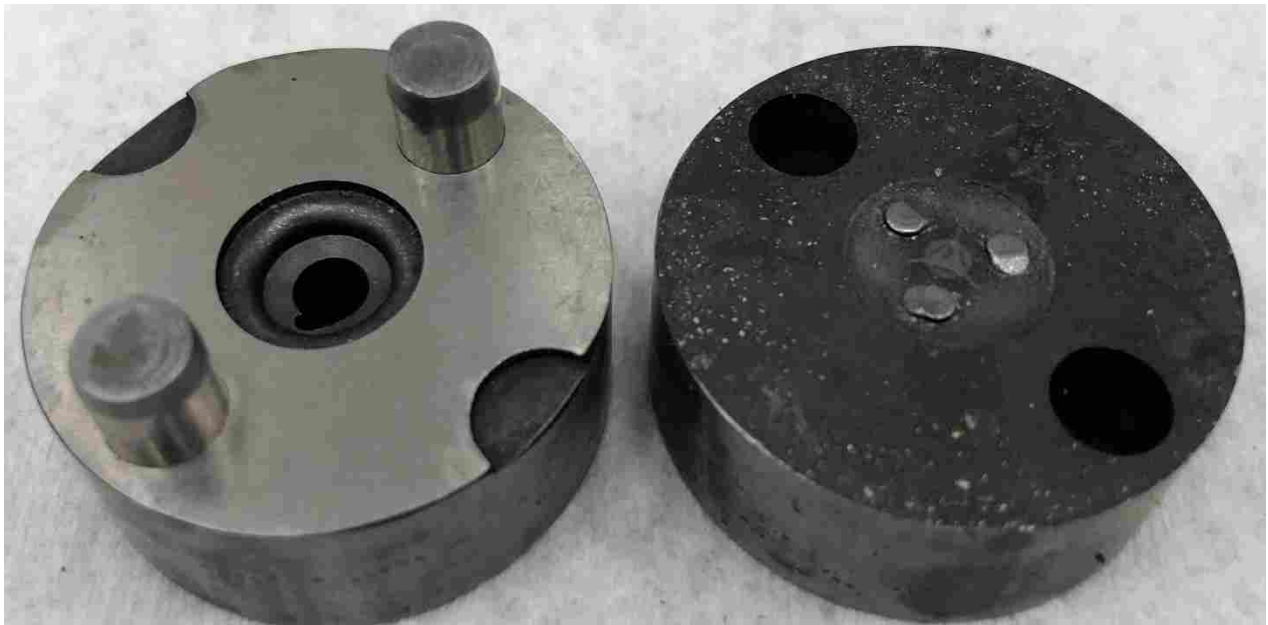
Figure 4-37: Dies for Pressing Drive Features into Bit Heads
