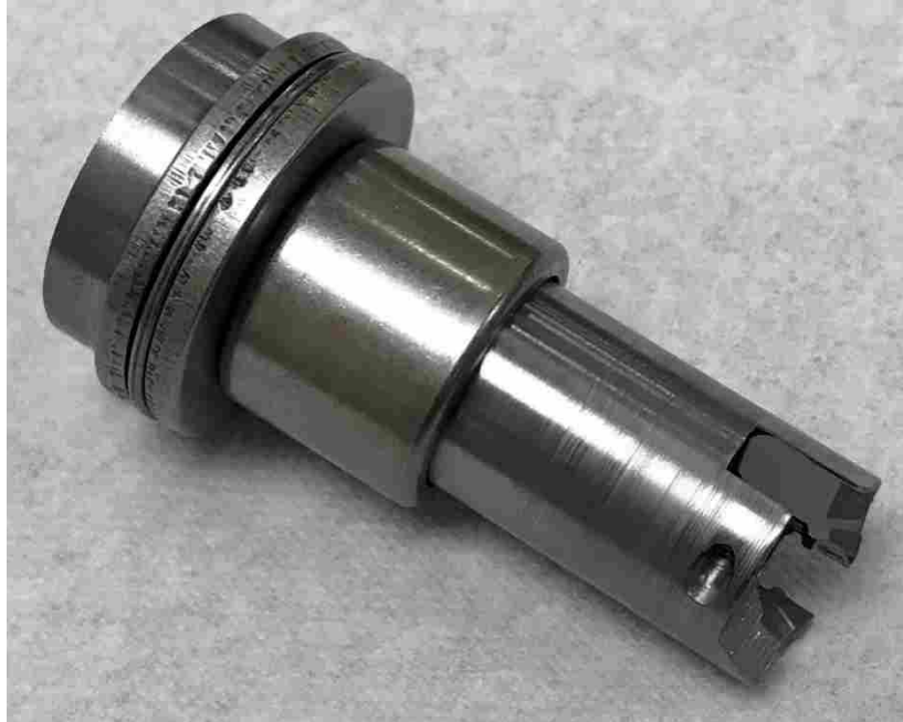
Figure 4-50: Cutter Assembly with Needle Bearing and Thrust Bearing
