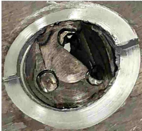
Figure 4-29: Severe Fracture of Bit Head
