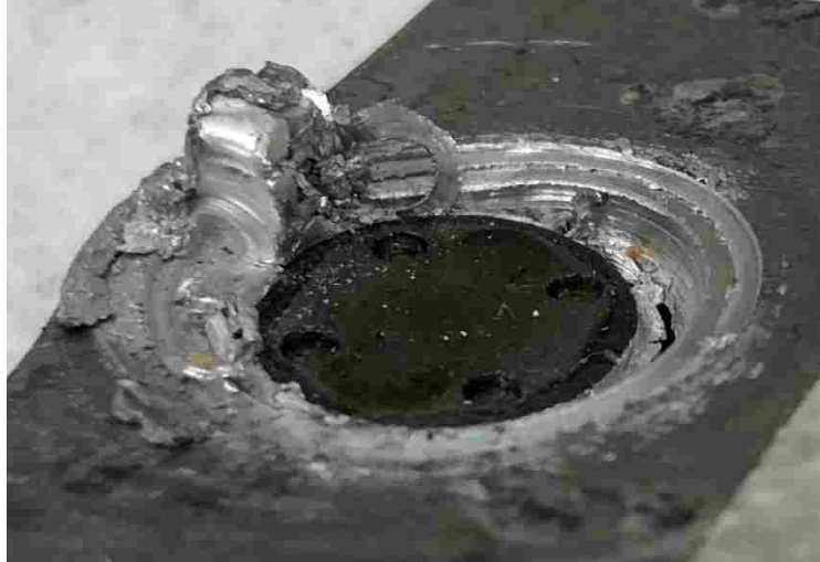
Figure 4-45: Aluminum Chip Build Up Due to Uneven Cutter Engagement
