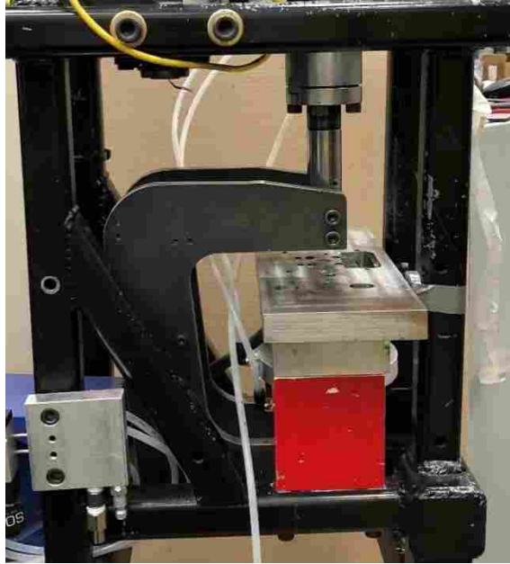
Figure 4-4: Pneumatic Clamp Side View
