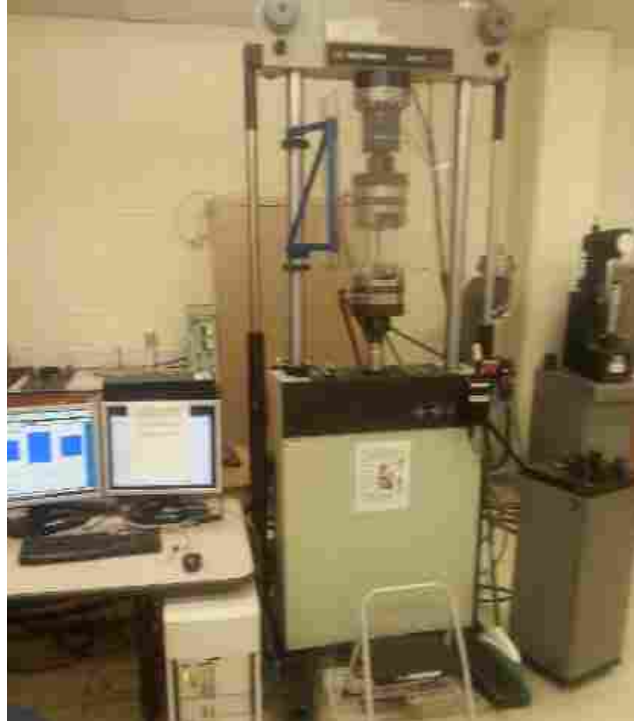
Figure 3-8: Hydraulic Instron for Fatigue Testing
