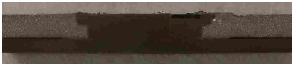
Figure 4-35: Unpolished Flush FBJ Cross Section
