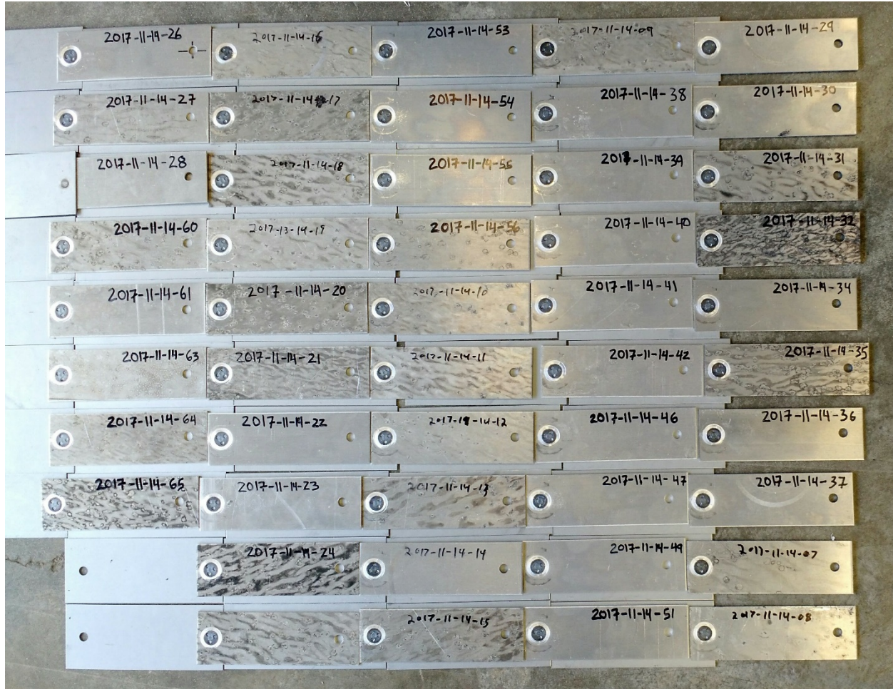
Figure 4-53: A Portion of the Samples Produced for the Corrosion Submission
