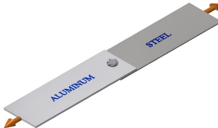
Figure 3-5: Lap-Shear Tension Configuration
