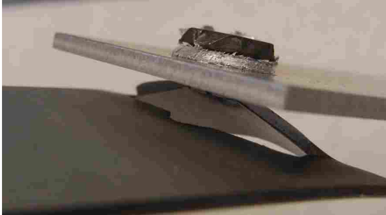
Figure 4-12: .5-5kN Fatigue Sample Weld Nugget Pullout Failure
