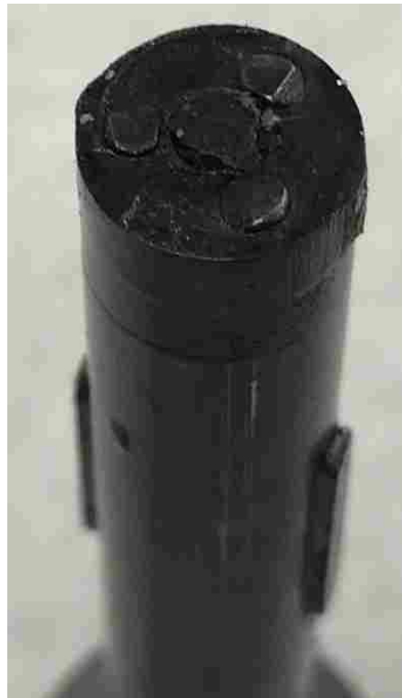
Figure 4-46: Flush Bit Driver After Several Hundred Welds
