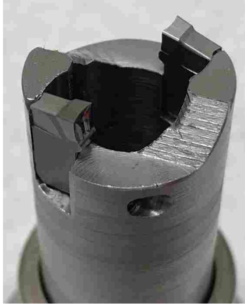
Figure 4-48: Flush Bit Cutter Assembly
