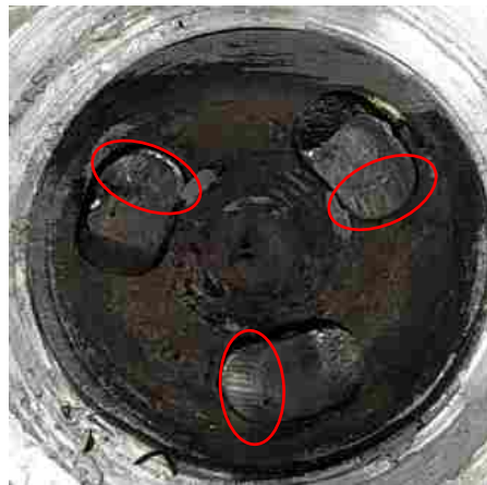
Figure 4-39: Less Common Stretching of Drive Features
