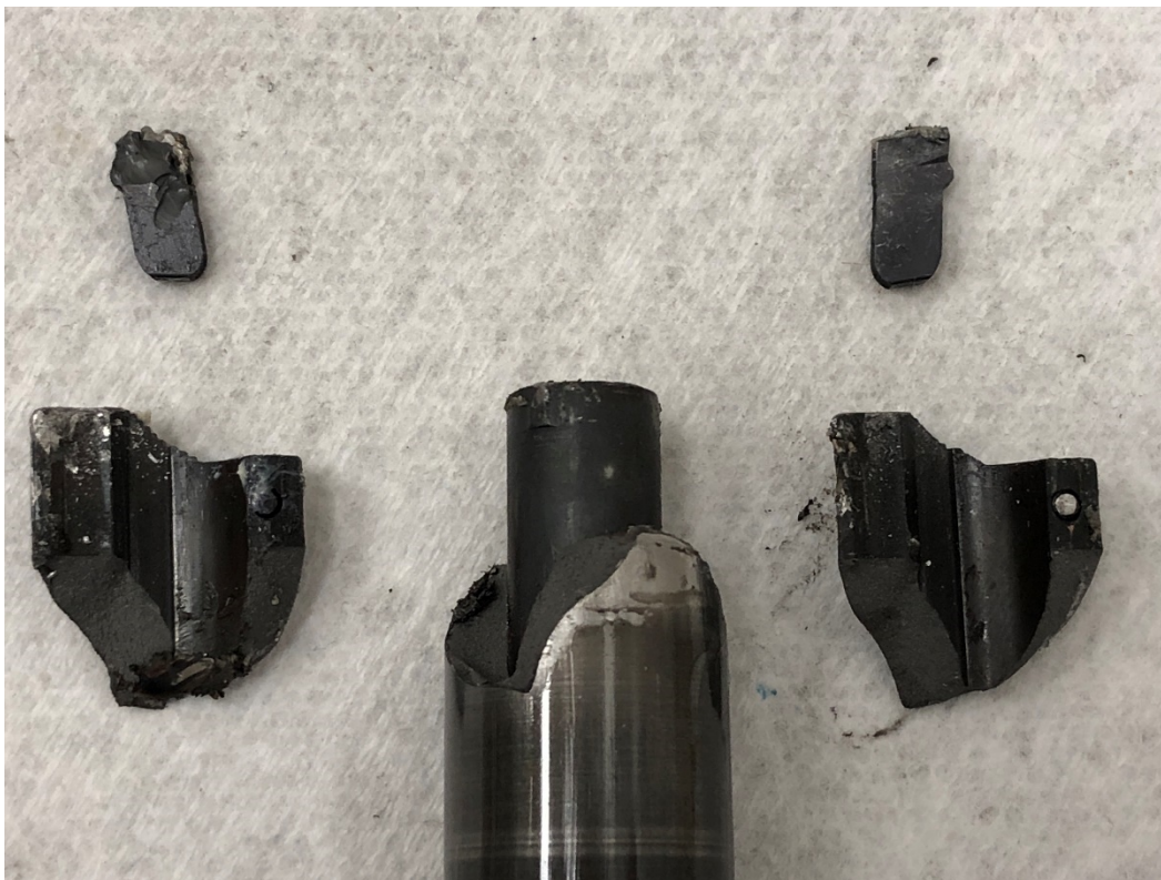
Figure 4-51: Broken Cutter After Bit Jammed In Clamp Block
