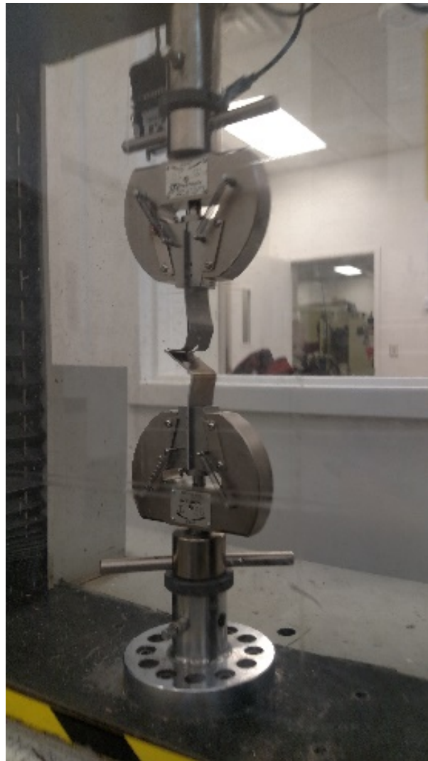
Figure 3-10 T-Peel Test as the Weld is Failing.
