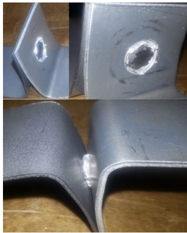
Figure 4-13 Material Joint Failure
