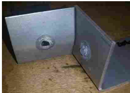
Figure 4-9 Nugget Joint Failure Small Steel Tear
