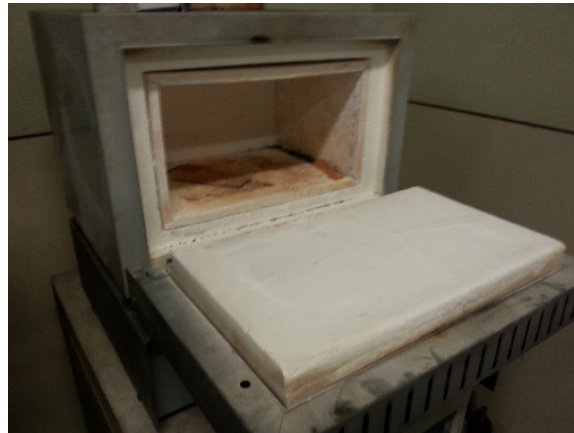
Figure 3-7 Oven for Warming Aluminum Coupon Before Bending
