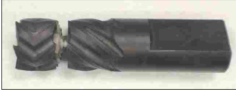
Figure 3-18: The BFSW End Mill After Heat Treatment
