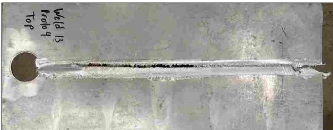
Figure 4-10: Typical Consolidation Success
