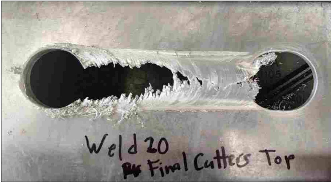
Figure 4-11: Weld 20 Test Result
