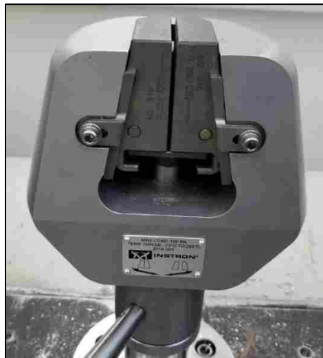
Figure 3-32: Instron Jaws for Lap Shear and T-Peel
