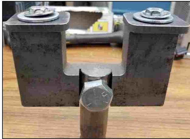
Figure 3-34: Instron Fixture for Cross Tension
