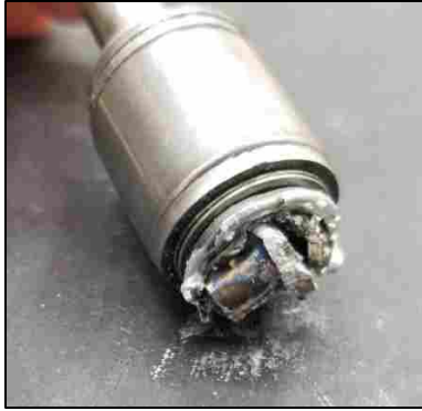
Figure 3-18: First Typical Bit-Driver Failure
