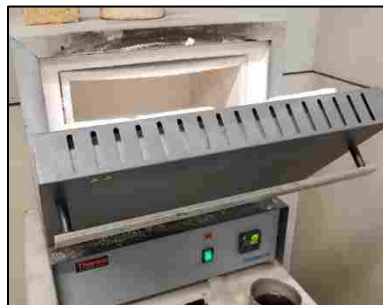
Figure 3-28: Oven for Pre-Heating Coupons
