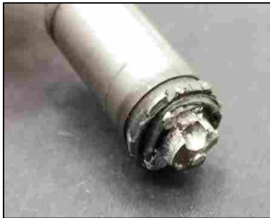
Figure 3-19: Second Typical Bit-Driver Failure
