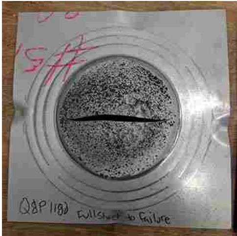
Fig 10-Biaxial Specimen Strained to Fracture Fig 11-Diagram of Samples Mounted in Bakelite
