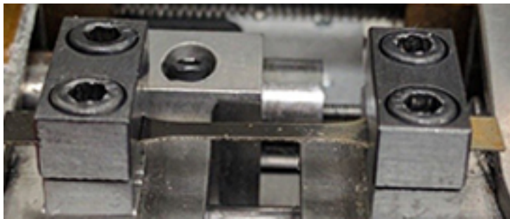
Fig 6-Micro-Tensile Specimen in the in situ Stage
