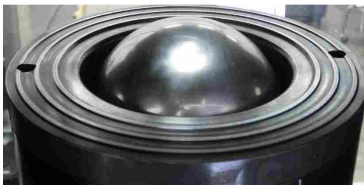
Fig 8-Tooling Used for Plane Strain and Biaxial Tension Experiments
