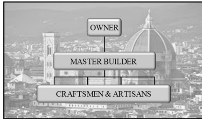
Figure 2-1: Contractual Relationships - Master Builder
