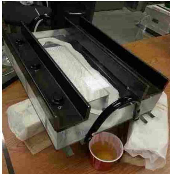
Figure 3-5: Second Tool with 3” Thick Acrylic
