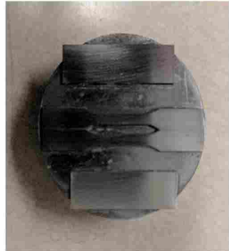
Figure 4-Micro-Tensile Specimens Mounted on a Steel Puck
