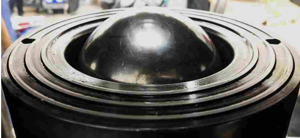
Figure 13-Tooling Used for Plane Strain and Biaxial Tension Experiments
