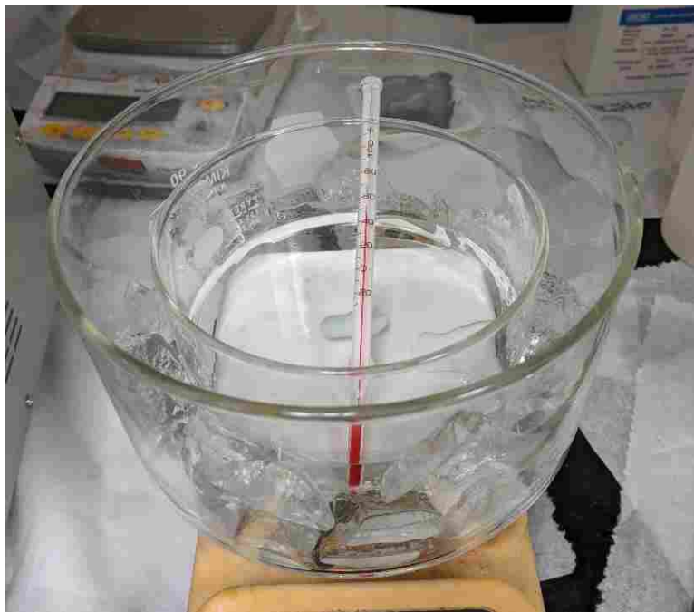
Figure 6-Preparing the Electrolytic Solution for Sample Polishing
