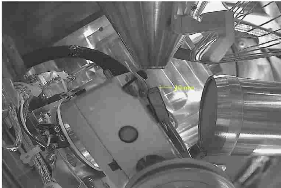
Figure 11-Image of the Tensile Stage in the Microscope with the EBSD Camera in Place
