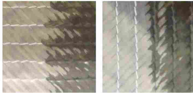
Figure 2-1: Dual-Scale Flow "Fingering": Along Stitching Fibers (Left) and in Between Tows (Right).
