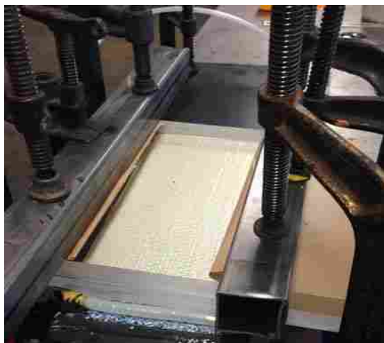
Figure 3-1: 1D Permeability Test Fixture
