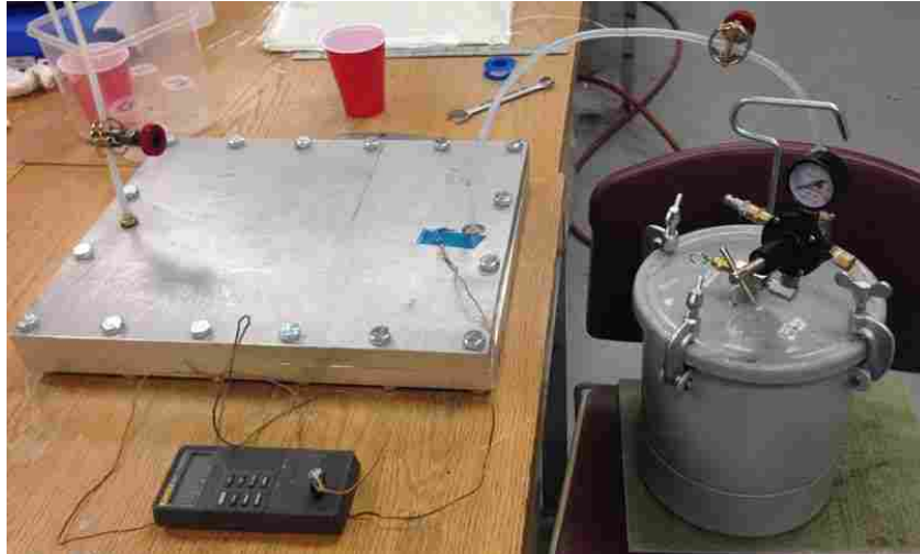
Figure 3-4: RTM Tool Configuration
