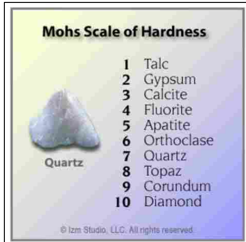
Figure 1-2: Mohs Hardness Scale
