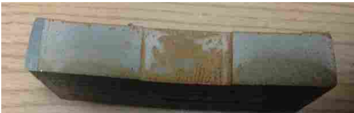
Figure 4-7: Specimen That Could Not Be Processed Because of Warping
