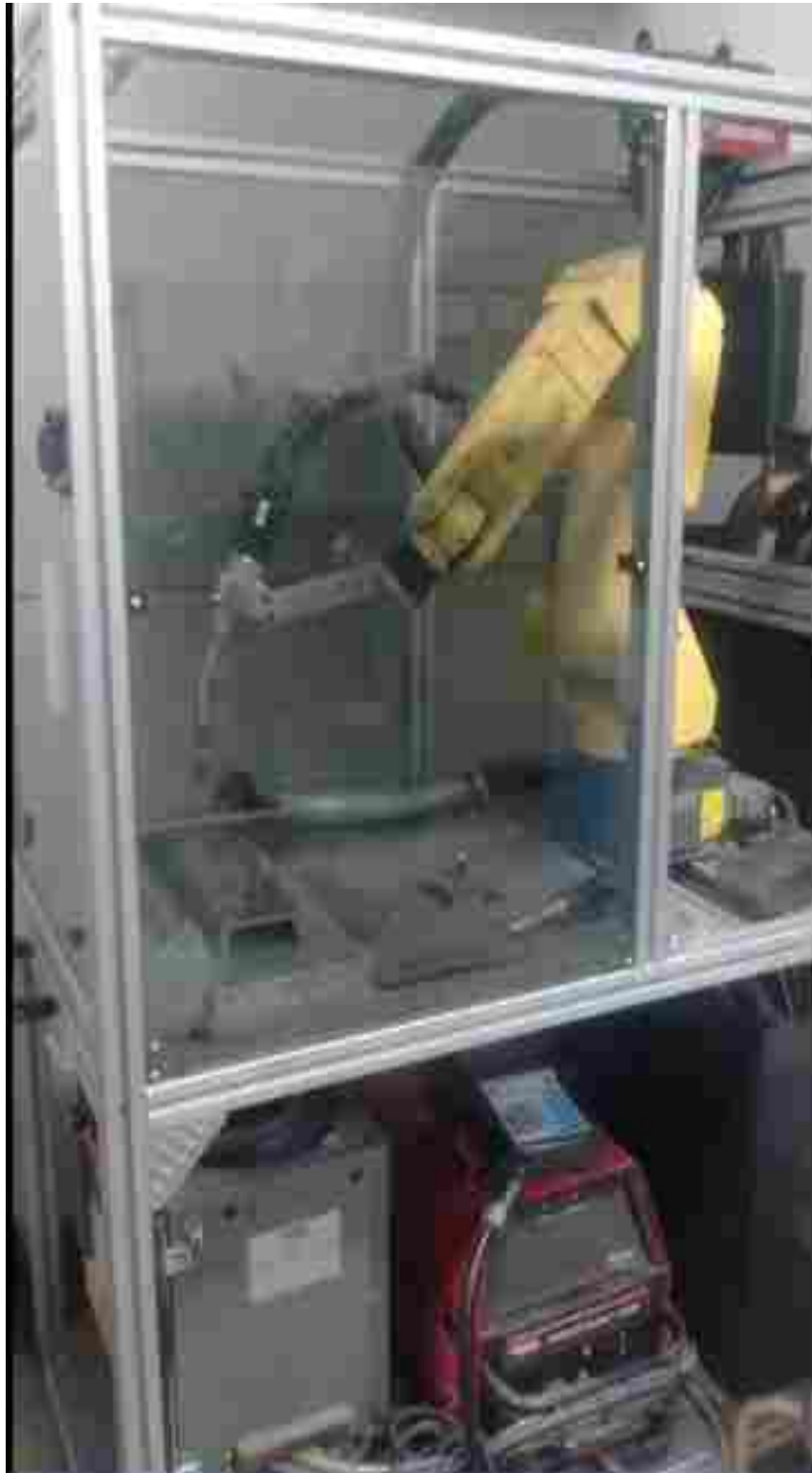
Figure 2-3: Robotic MIG Welder
