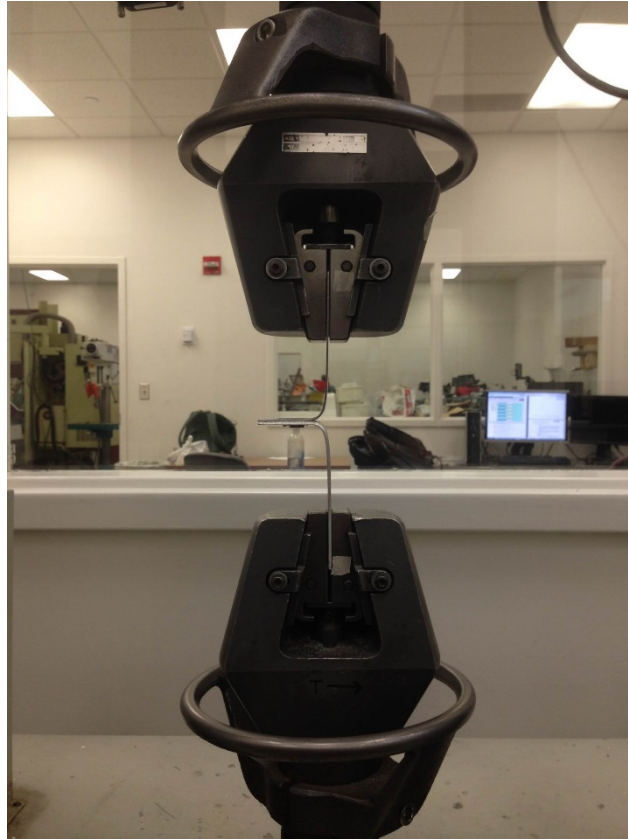
Figure 3-16: Peel Testing Specimen in Instron Machine
