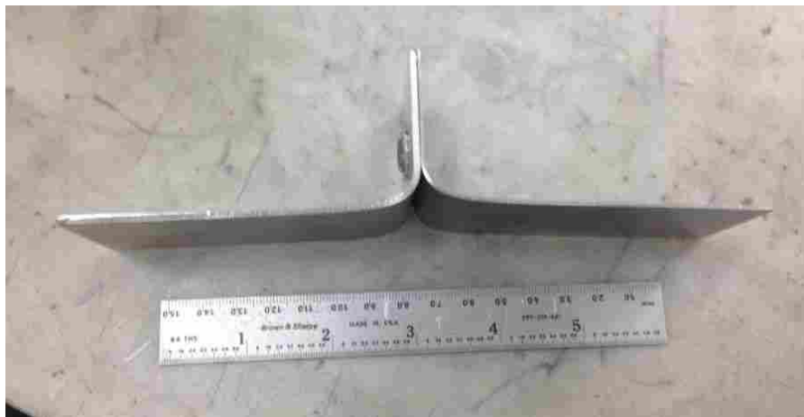
Figure 3-15: Bent Peel Testing Specimen
