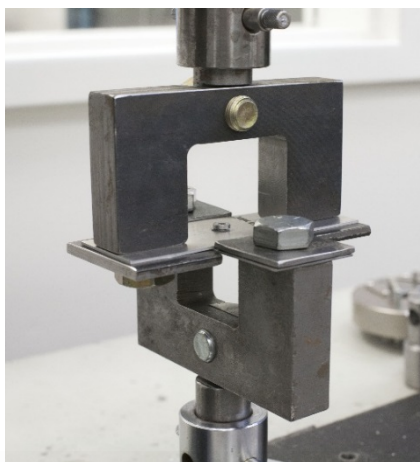
Figure 3-13: Cross-Tension Testing Fixture with Specimen Placed
