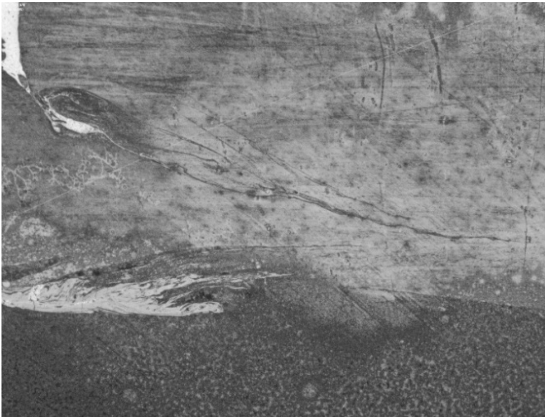
Figure 4-8: Micro-Cracks in Sectioned Weld
