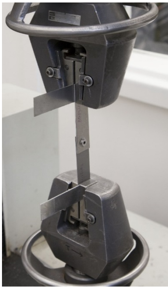
Figure 3-11: Lap-Shear Tension Testing in Instron
