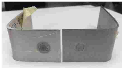
Figure 4-7: Peel Testing Interfacial Failure
