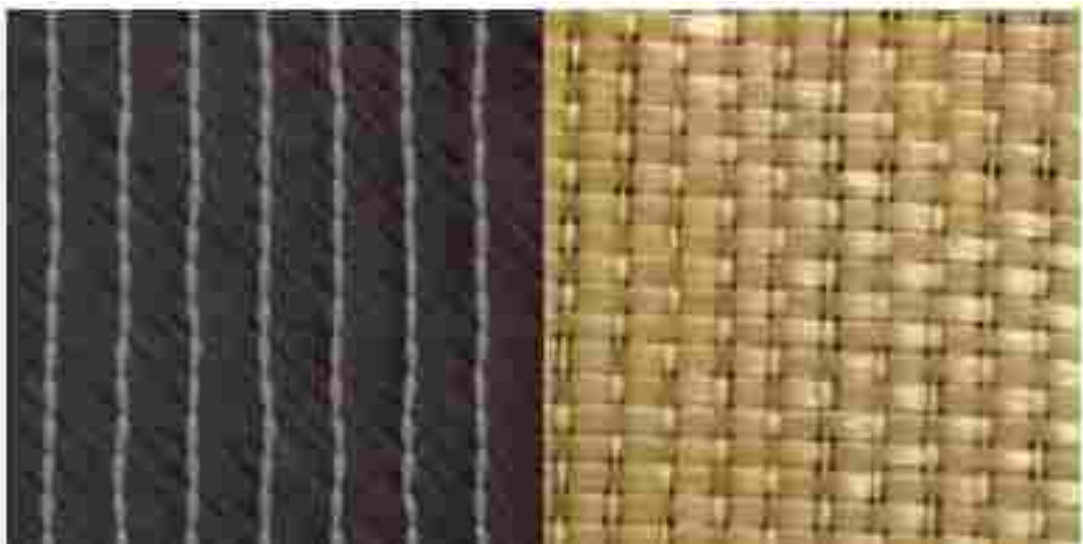
Figure 3-1: Vectorply Carbon Fiber (left) and JB Martin Fiberglass (right) Samples
